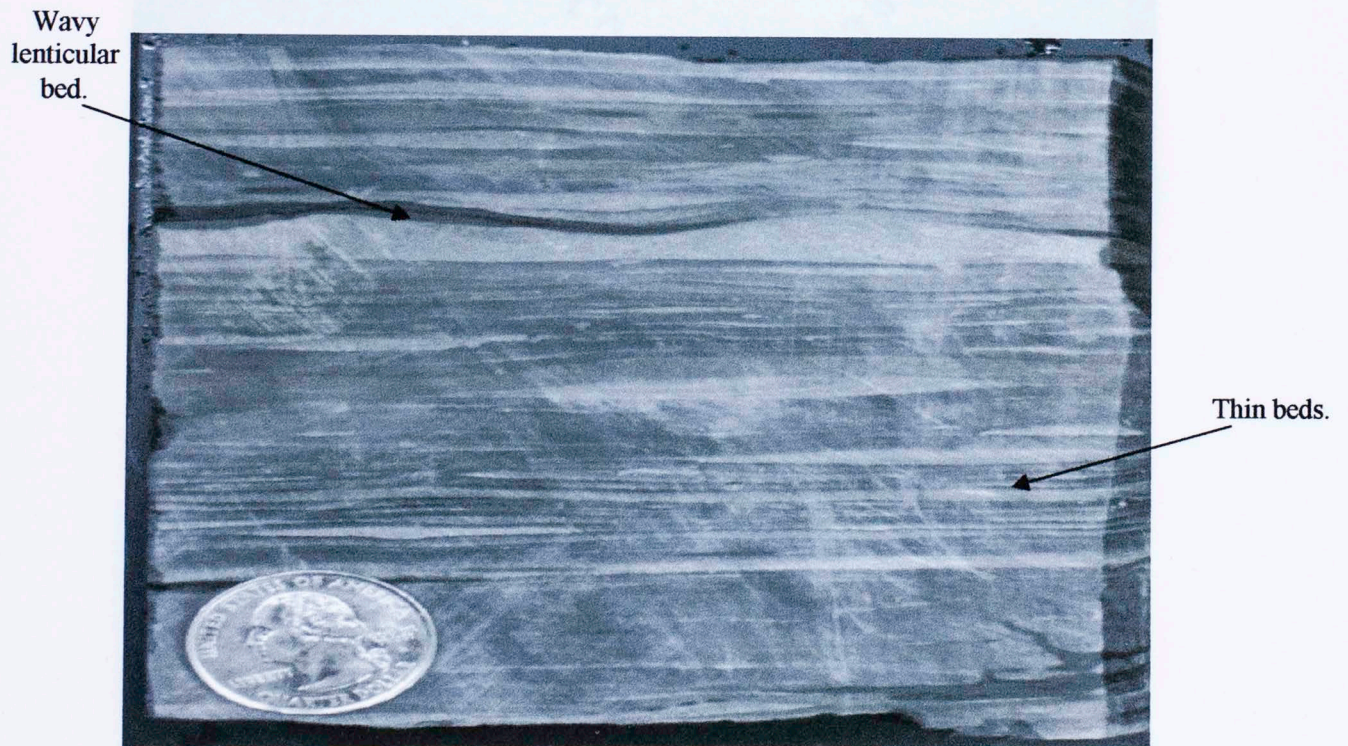
Figure 3.17-Shale with 0.2 to 0.4 inch thick, interbedded siltstone lenses that contain planar, wavy, and lenticular features. Depth is 14,085 feet, Hunt
