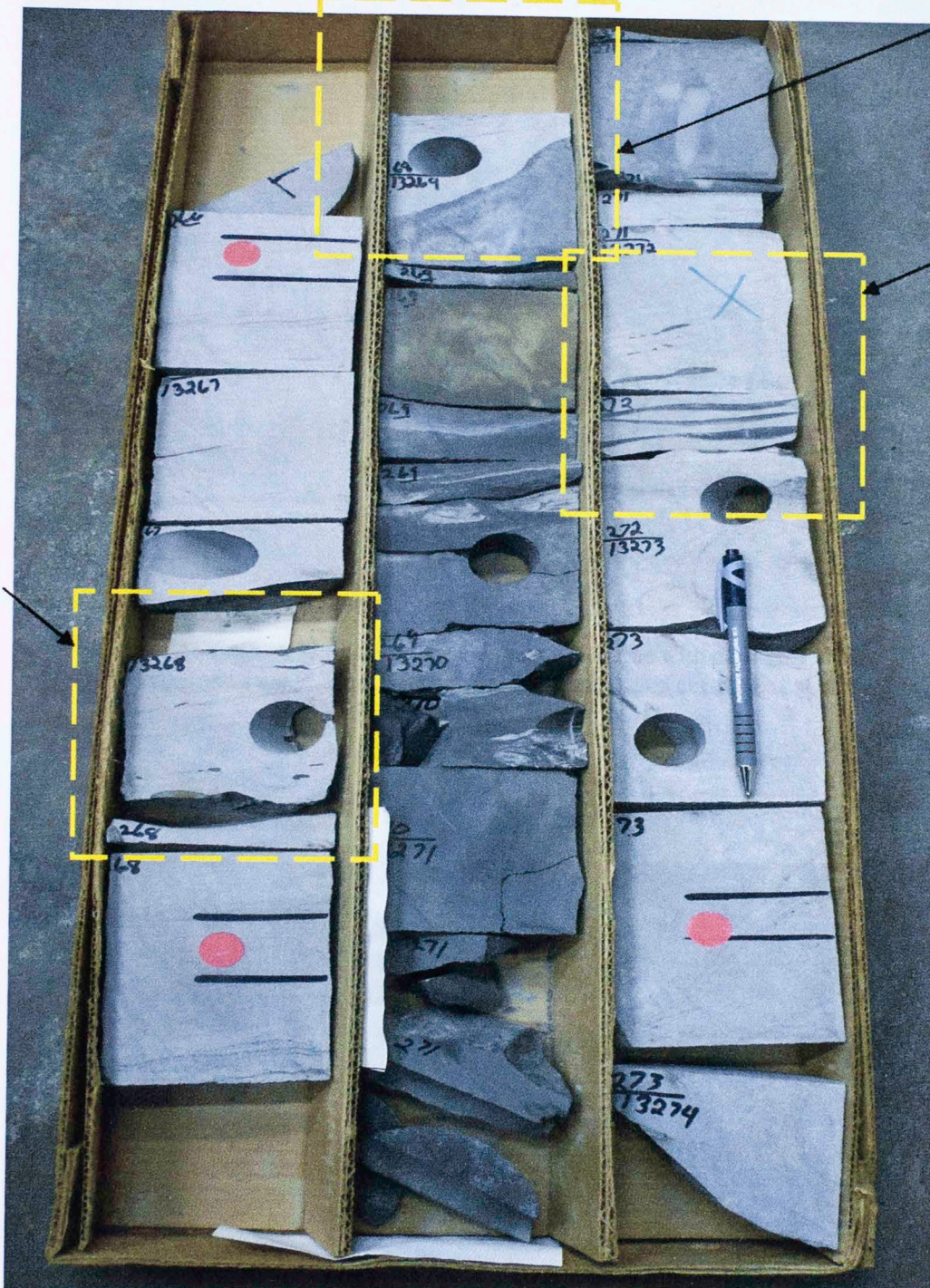
Figure 3.26-Dark shale between two sandstone intervals. Depth is 13,277 to 13,270 feet, Amoco Smith Unit 1.
