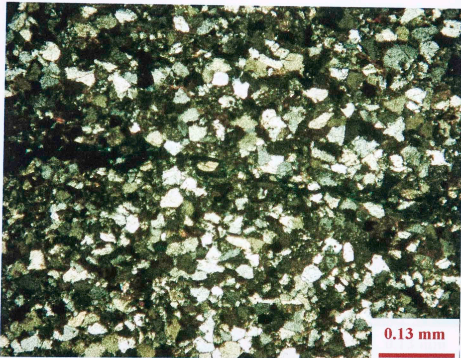
Figure-3.36 Hunt Gillingham #1 Depth: 14,096.15' Magnification: 40x Plane polarized light (above) Cross polarized light (below) Very fine sandstone with dissolution creating a migratory pathway.
