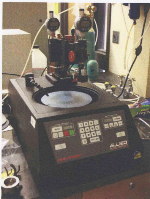
Figure 13: Allied Multiprep polisher. This technique delivers smooth and parallel sample surfaces due to continuous motion of the sample and disk and precise alignment of motion system.
