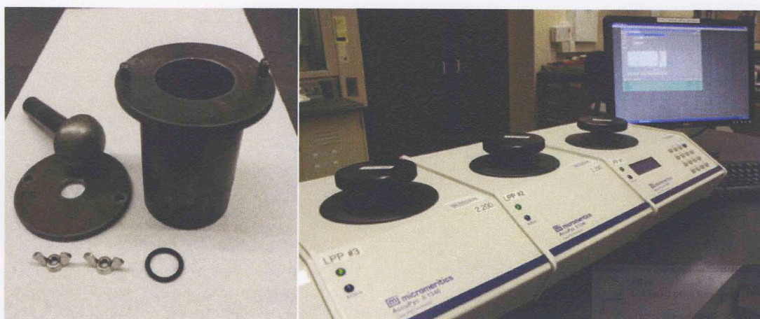
Figure 11: Equipment for shale porosity measurement. (Left) Crushing vessel for powdering shale. (Right) Micrometrics low pressure pycnometer for measurement of grain volume and grain density.
