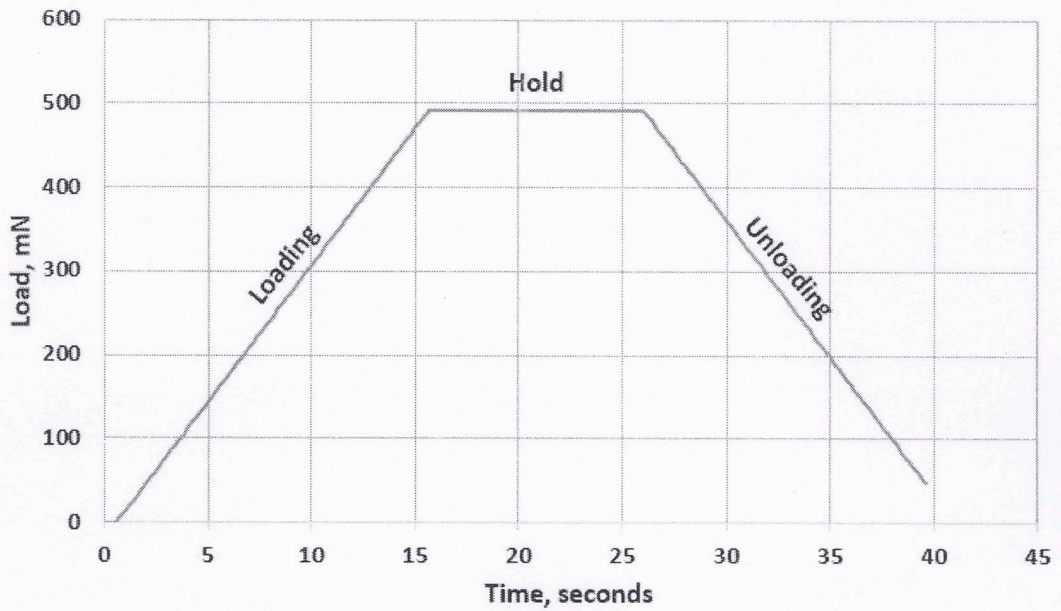
Figure 29: Variation of load versus time during a single nanoindentation test on a shale sample. Peak load threshold was set to 500 mN.
