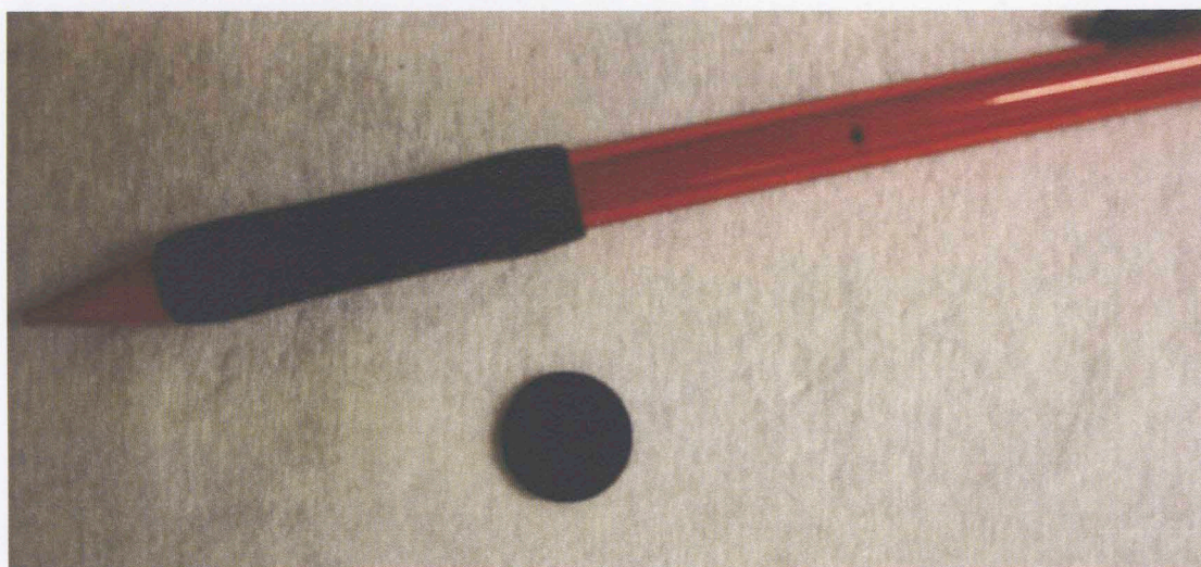
Figure 102: Disc of organics prepared by pressing the organic recovered from dissolving organic rich shale in HCl and HF. Diameter of the disc is 1 cm while thickness is 1 mm.
