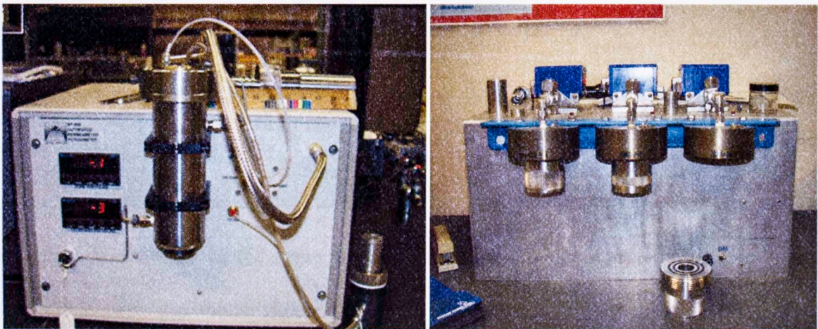
Figure 3.1: AP608 (left) and HPP (right) equipments used to measure porosity.
