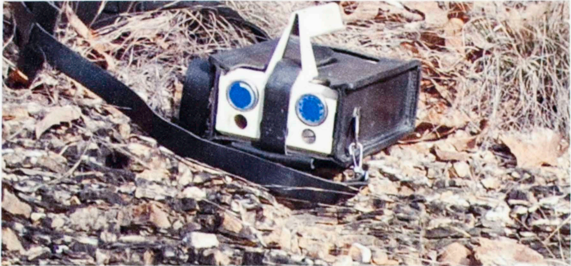
Figure 6 Scintrex GRS-500 hand-held detector used to create outcrop gamma-ray logs.
