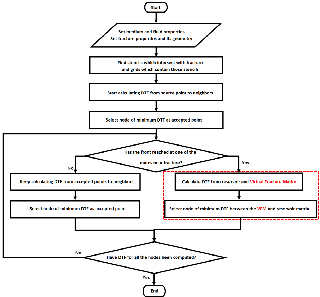
Figure 5.6: Flow chart for Embedded Fracture MFM with VFM.
