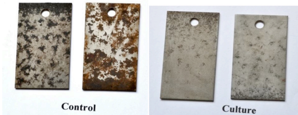
Figure 2.4 (Left) pre-oxidized coupons incubated in media and (right) after incubated with G. sulfurreducens and S. oneidensis cultures incubated in media for 3 weeks (Starosvetsky, 2016).
