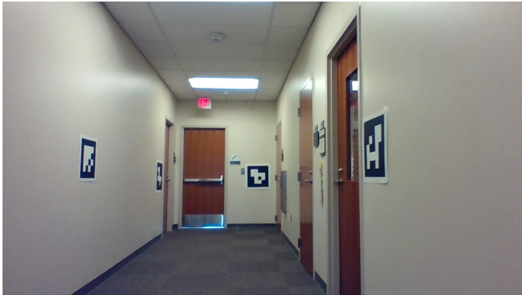
Figure 4.9 ArUco markers' placement in the corridor
