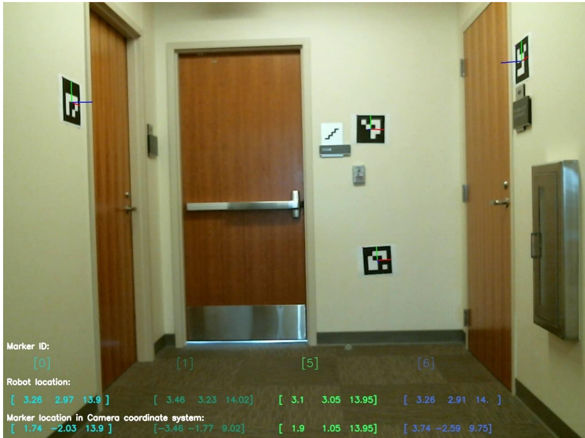
Figure 4.10 Localization in the corridor using ArUco markers. Locations of all the markers in camera coordinate system and estimated robot locations are displayed below the marker IDs.
