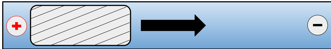
Figure 6.2: Representation of a Galinstan slug in an electrolyte solution with an applied voltage potential
