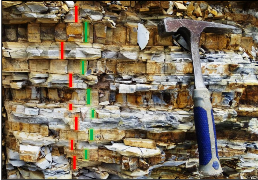
Figure 98. Picture taken around foot 20 at the I-35 outcrop, showing abundant and well developed vertical fractures in hard beds (green lines) which generally terminate against soft beds (red lines).
