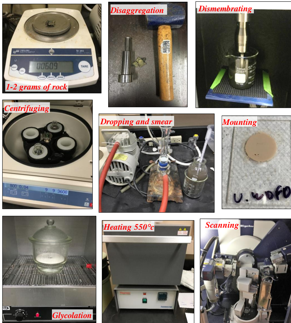
Figure 13. Collages of pictures of the actual procedure followed to prepare samples for clay-size XRD analysis.
