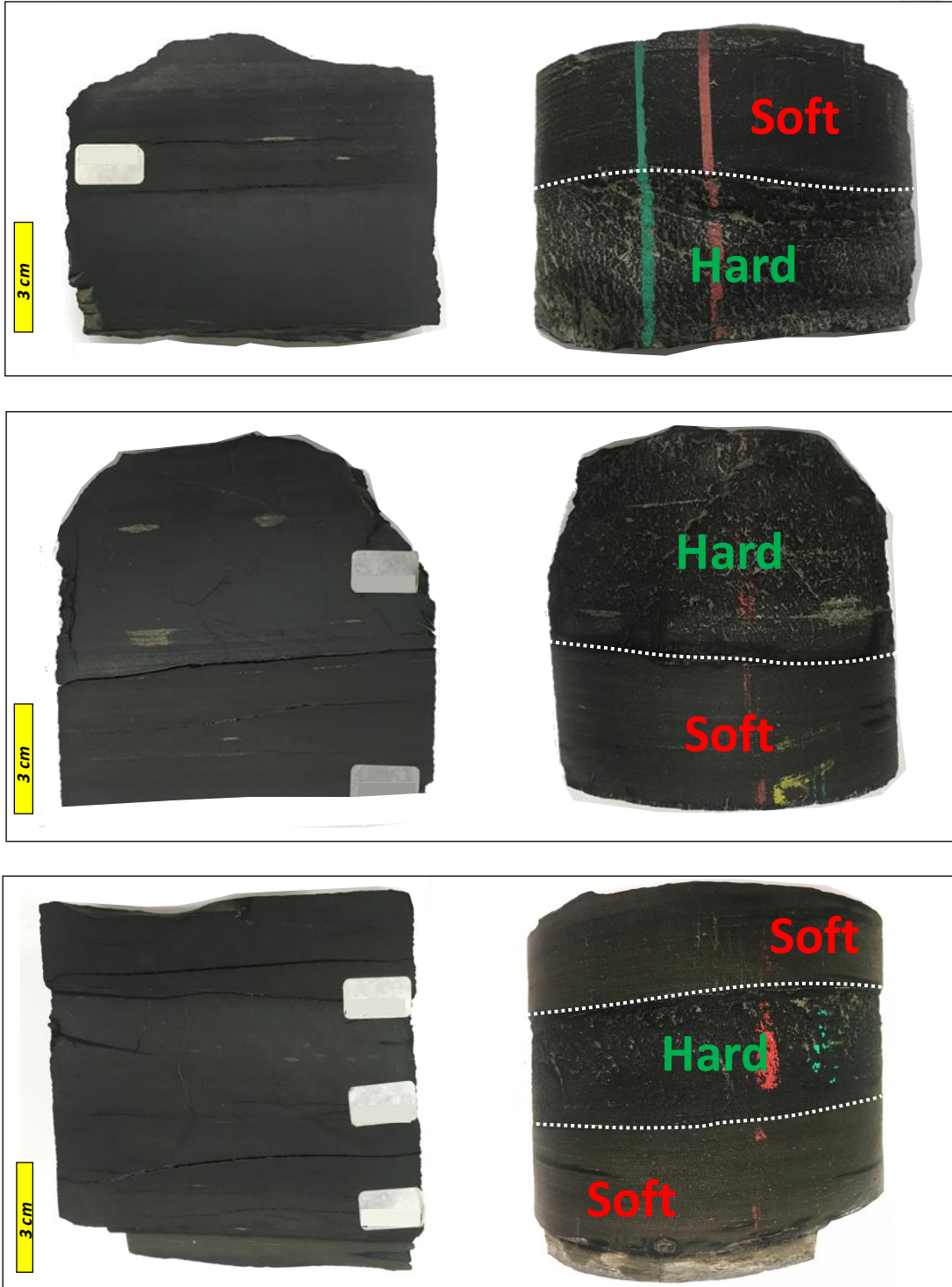
Figure 108. Examples of subtle changes in the back side of a Woodford Shale core that can help to distinguish soft and hard beds. Courtesy of Richard Brito.
