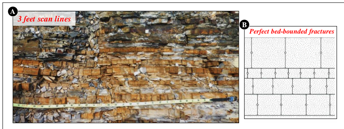
Figure 11. Outcrop picture showing methodology conducted for the fracture analysis. (B) Sketch showing the type of fractures described in this study: bed-bounded fractures (Gale et al., 2014)
