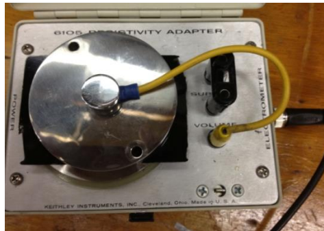
Figure 3.11: Electrical conductivity measurements for highly resistive specimens.
