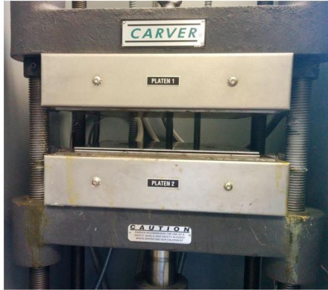
Figure 2.2: Photograph of the sample fabrication inside preheated carver press.
