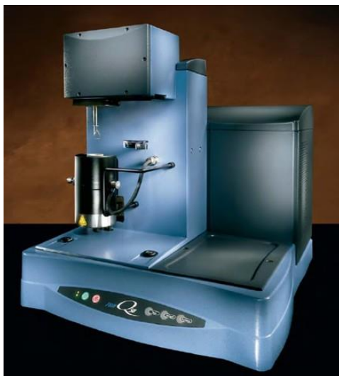
Figure 3.1: TA instrument Q-50 model used for TGA tests.
