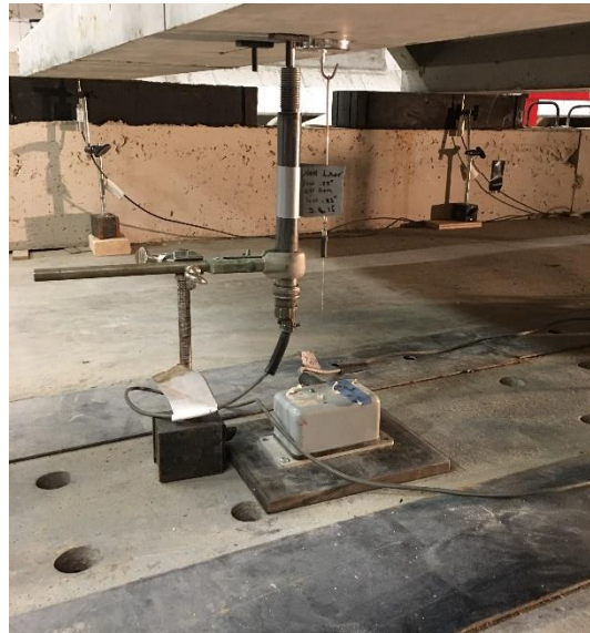
Figure 154: Deflection measurement under load point showing LVDT and wire pot (note tabs remaining for attachment of BDI strain gauge on girder)
