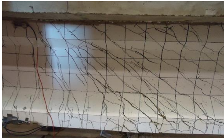
Figure 41: Test C1 failure, note large shear cracks and horizontal cracks in bottom flange
