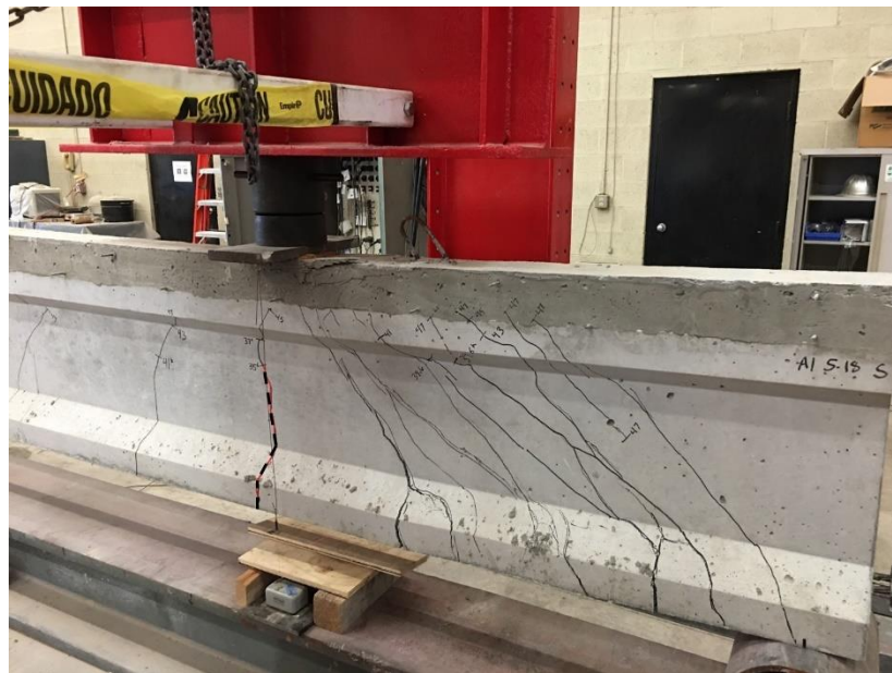
Figure 88: Test A1s cracking with initial cracks marked with red dashed lines
