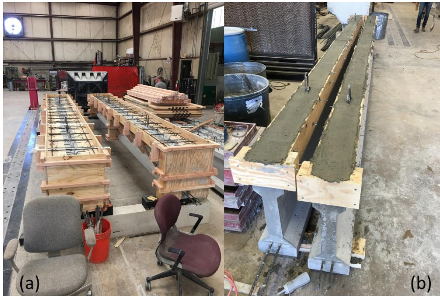
Figure 64: Girder C replica formwork (a) and girder A replicas with fresh concrete (b)
