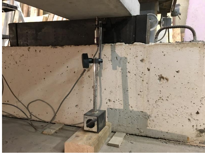
Figure 153: LVDT positioned to measure deflection at bearing
