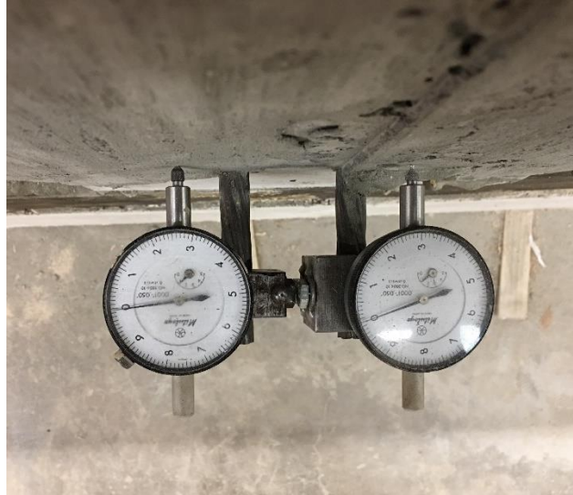
Figure 84: Dial gauges used to monitor strand slip
