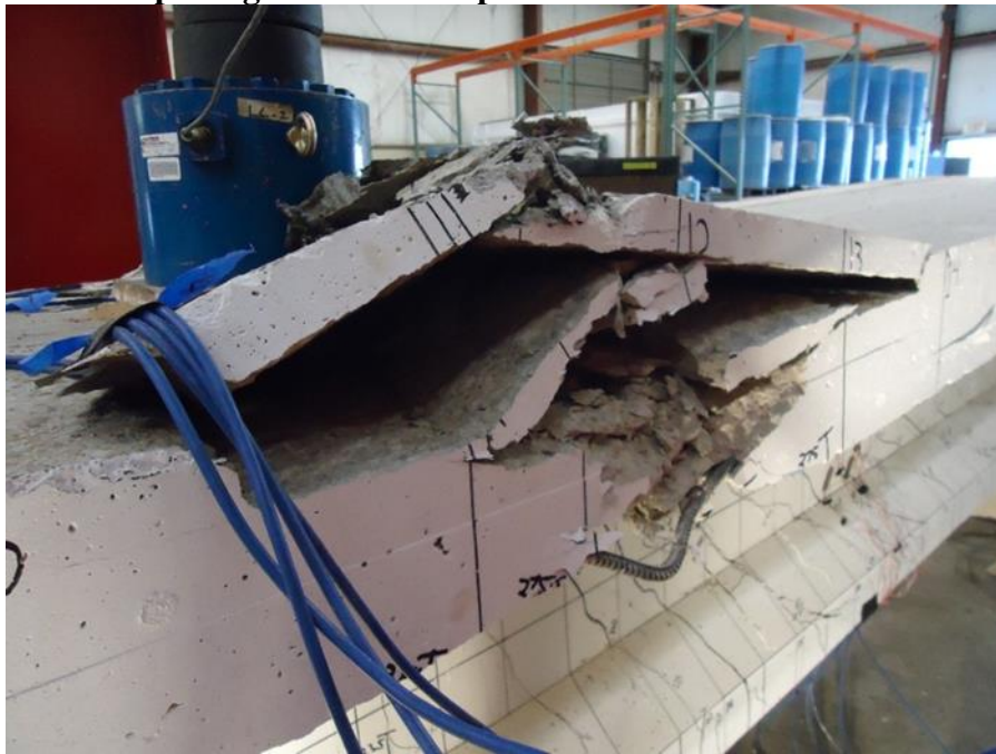
Figure 51: Crushing in girder deck and buckling of reinforcing steel
