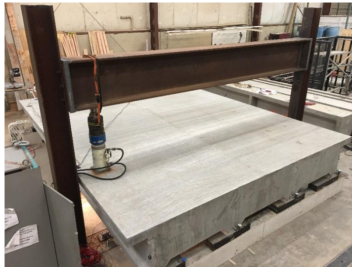
Figure 150: Scale bridge with load set up shown
