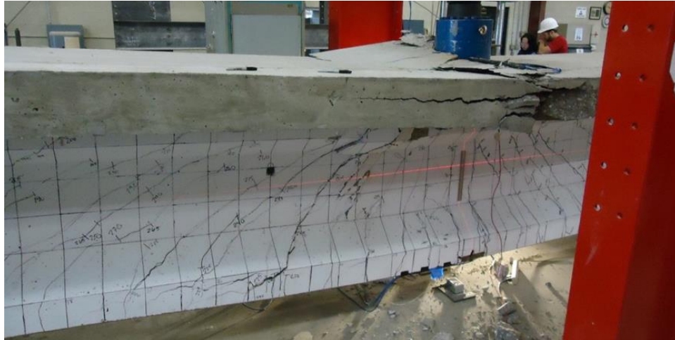
Figure 50: Test C2 failure, showing a large shear crack in the center of the image that entered the top flange where a compression failure occurred
