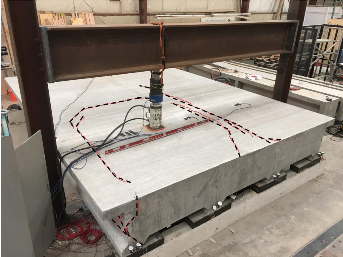
Figure 110: Cracking in scaled bridge section slab at failure (highlighted in red and black for clarity)
