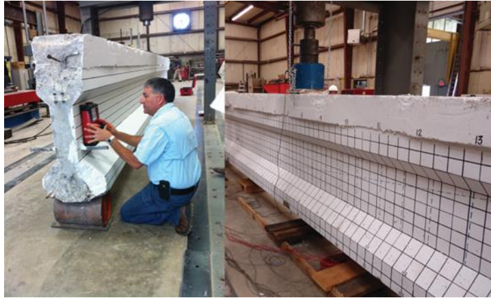
Figure 18: Mr. Matt Romero using ground penetrating radar to locate reinforcing bars in girder A (left), and finished reference grid showing steel locations for girder A (right)
