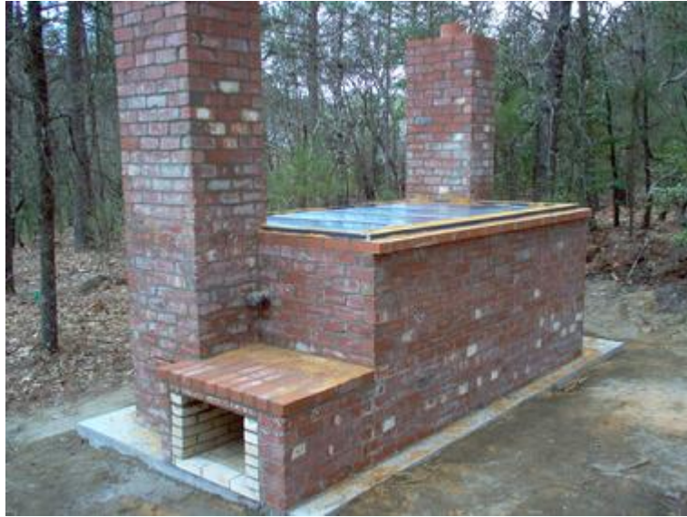
Figure 1 – An Adam Retort. Retrieved online 3/17/2012 from http://terrapreta.bioenergylists.org/content/freefarm-adam-retort
