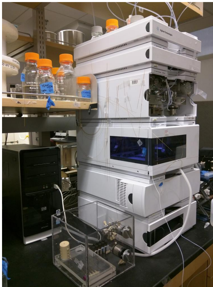
Figure 3-15 Comparison of prototype of microHPLC and a commercial HPLC (Agilent 1200).
