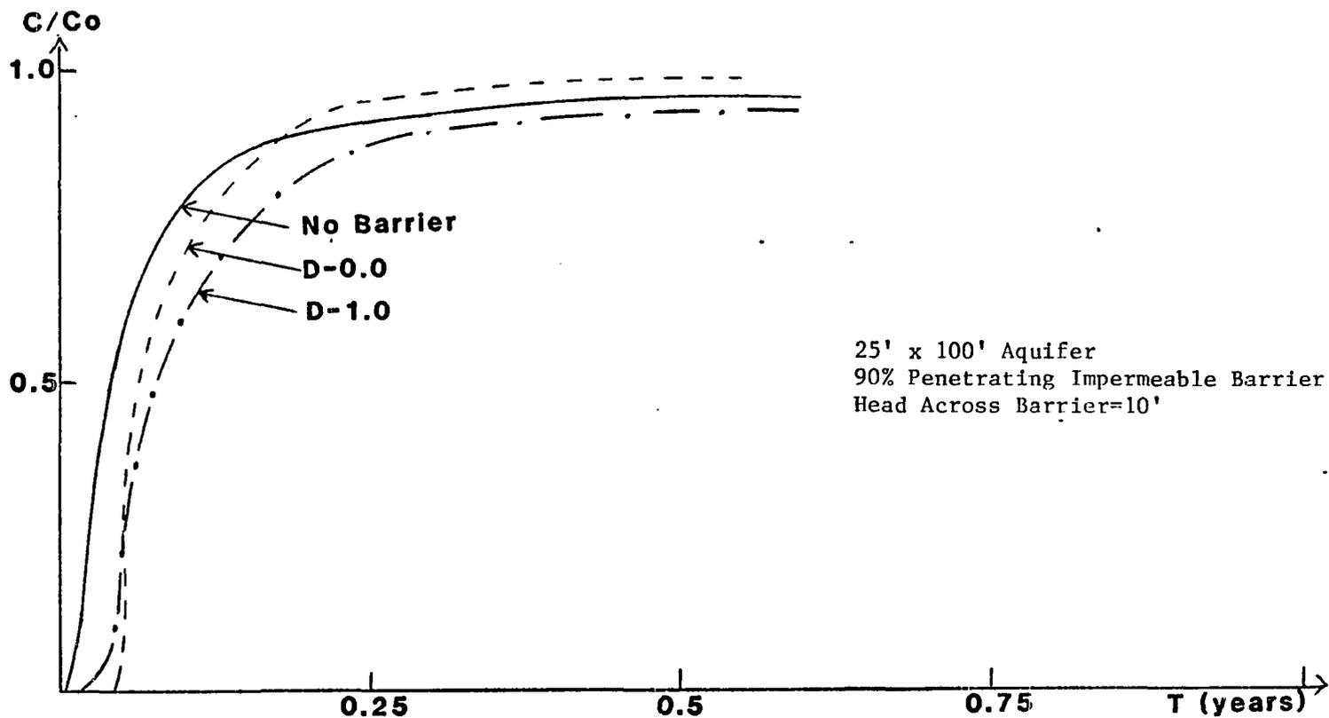
Figure V-19: Pollutant Breakthrough Curves in 25 Foot Deep Aquifer for Head Difference Comparable to 100 Foot Deep Aquifer.
