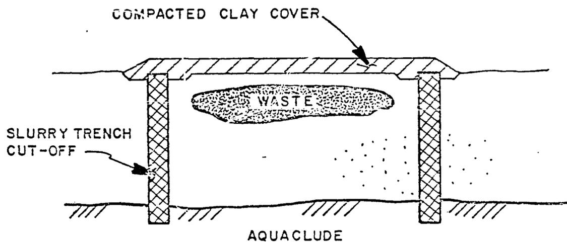
Figure III-3: Isolation of Existing Buried Waste (Ryan, 1980).
