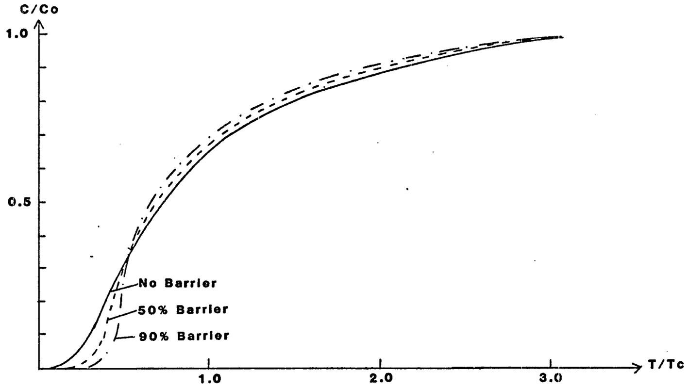
Figure V-5: Pollutant Breakthrough Curves for Aquifer Subjected to 3/4 Recharge.
