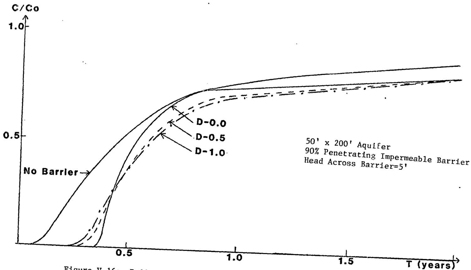
Figure V-16: Pollutant Breakthrough Curves for 50 Feet Deep Aquifer.
