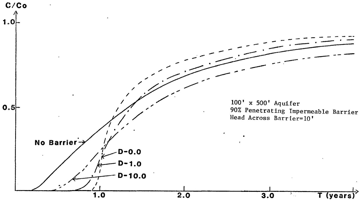
Figure V-21: Pollutant Breakthrough Curves for an Elongated Aquifer.
