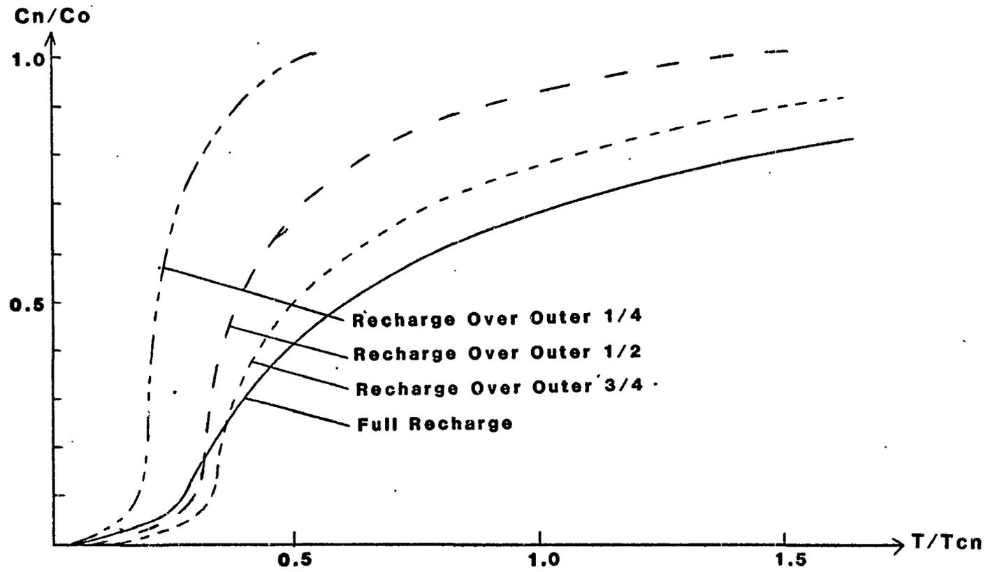
Figure V-10: Pollutant Curves for 90% Penetrating Barrier at Constant Amounts of Recharge.
