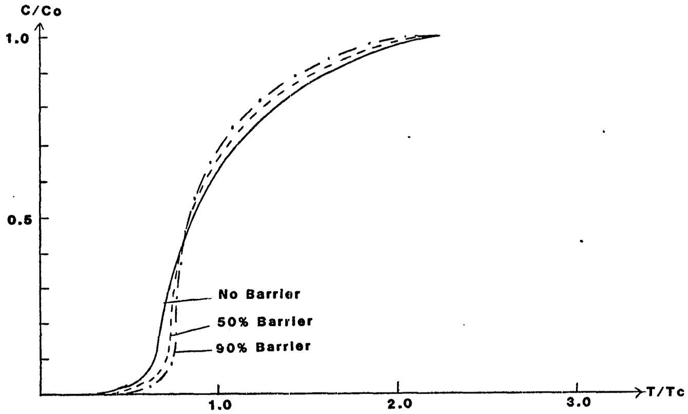
Figure V-7: Pollutant Breakthrough Curves for Aquifer Subjected to 1/4 Recharge.
