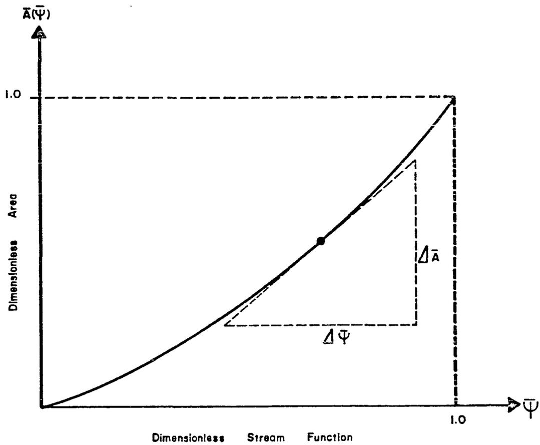
Figure IV-3: Idealized relationship indicating the total dimensionless area swept out by a given dimensionless streamline (McLin, 1980).
