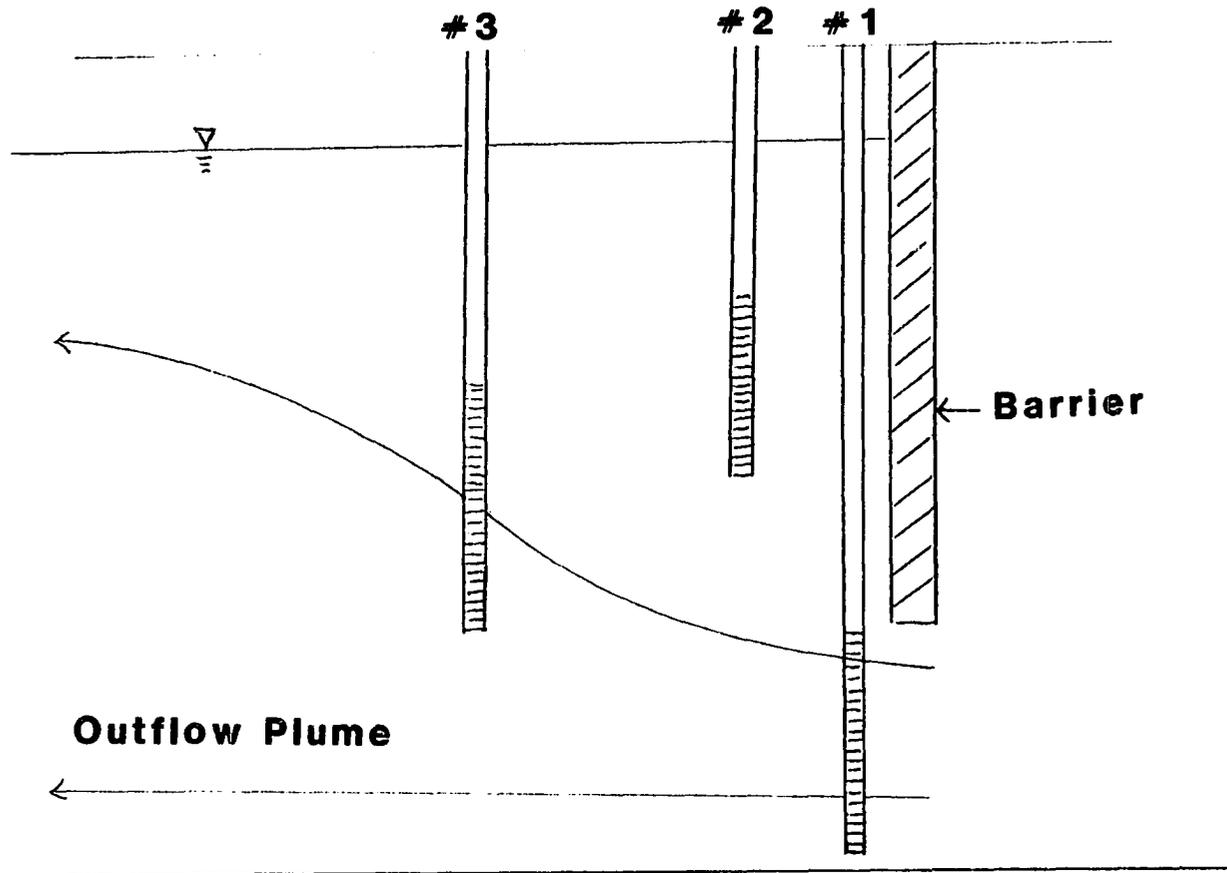
Figure V-28: Well Locations Outside An Imperfect Barrier.
