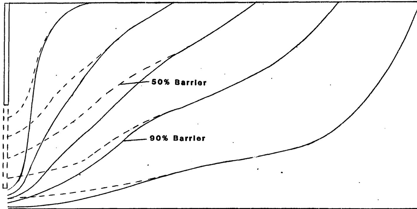
Figure V-4: Streamline Distributions for 50% and 90% Penetration Barrier.
