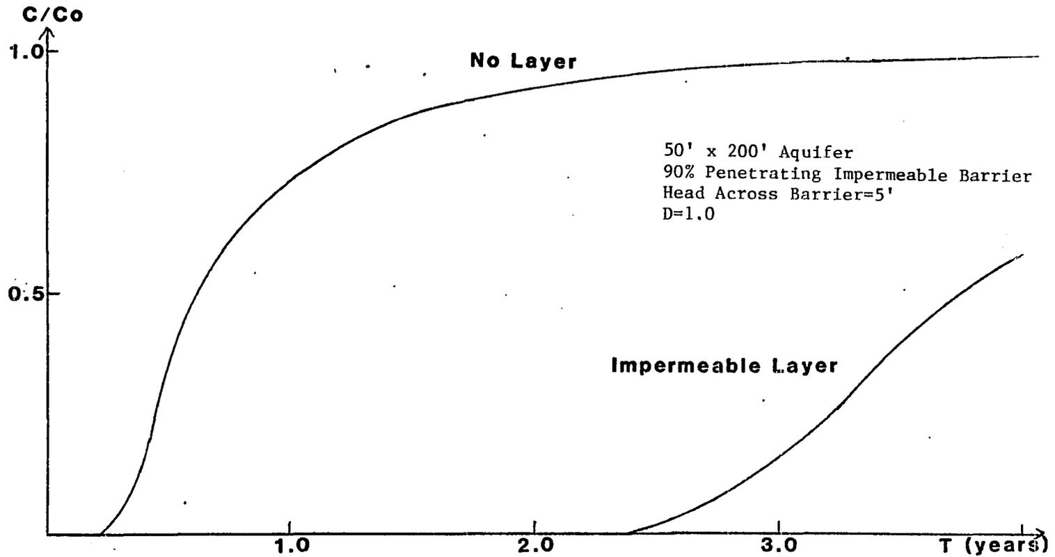
Figure V-23: Pollutant Breakthrough Curve for Barrier Keyed to Impermeable Layer (50 foot).
