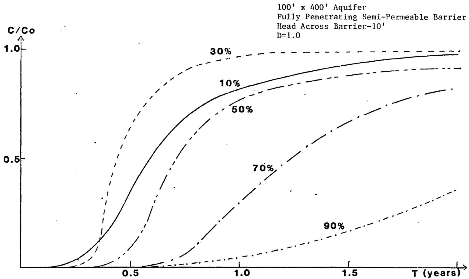
Figure V-24: Pollutant Breakthrough Curves at Selected Depths Adjacent to a Semi-Permeable Barrier.
