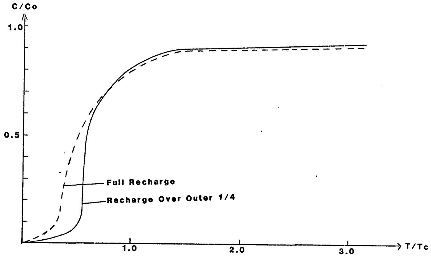
Figure V-13: Pollutant Breakthrough Curves for 90% Penetration Barrier in Horizontally Conductive Soil Under Variable Recharge Lengths.
