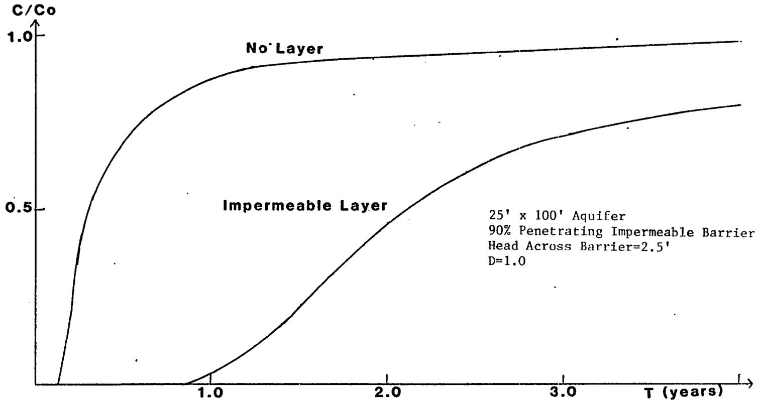
Figure V-22: Pollutant Breakthrough Curves for Barrier Keyed to Impermeable Layer (25 foot).
