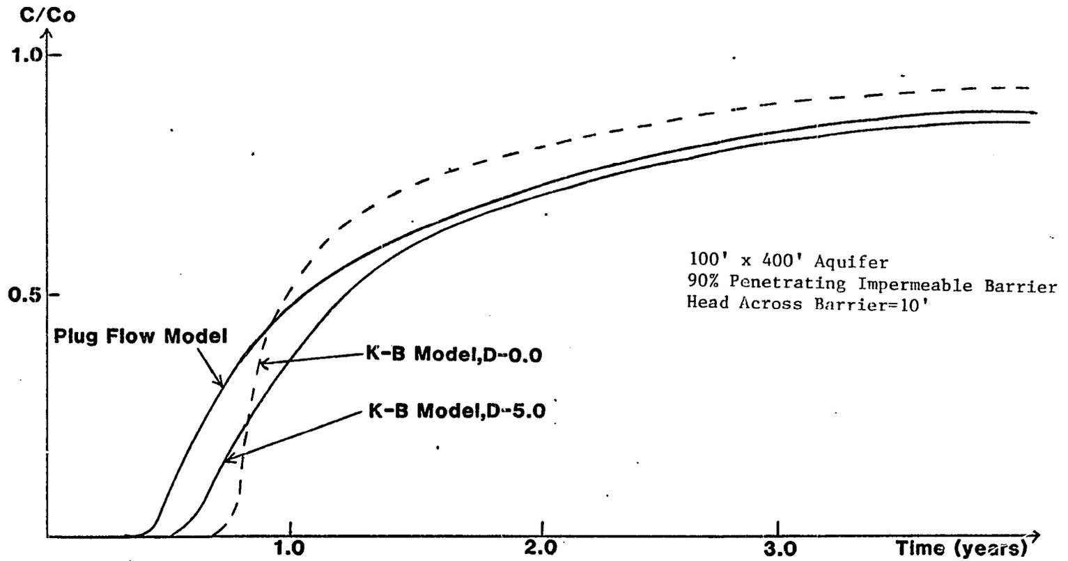
Figure V-27: Comparison of Simple and K-B Models.
