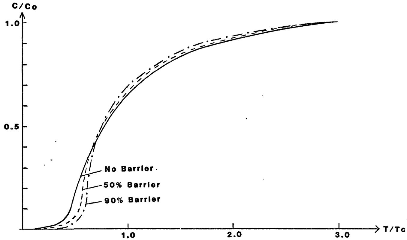
Figure V-6: Pollutant Breakthrough Curves for Aquifer Subjected to 1/2 Recharge.
