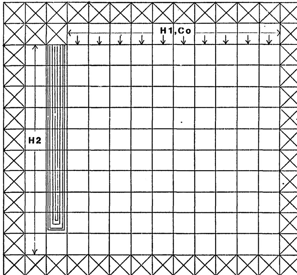
Figure V-14: Grid Representation of Aquifer Subjected to Contaminated Recharge.
