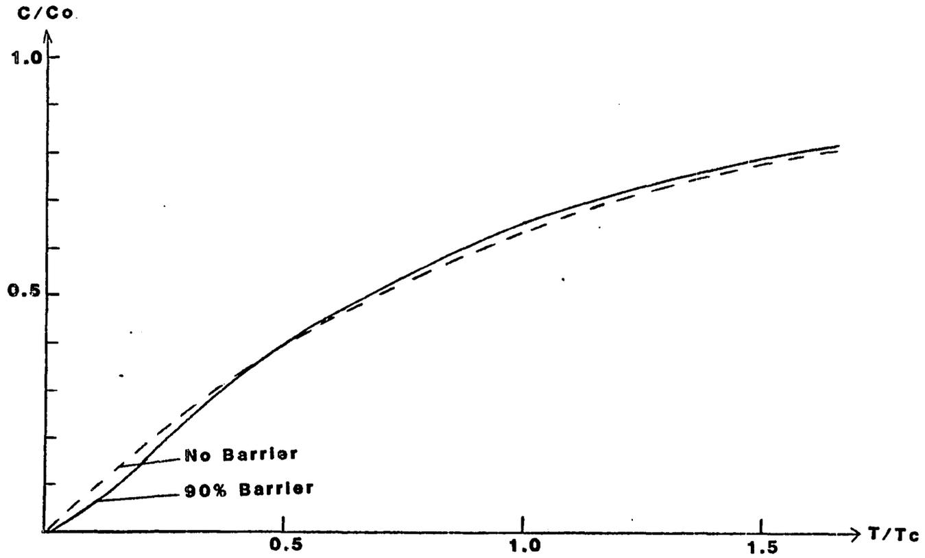
Figure V-12: Pollutant Breakthrough Curves for No-Barrier and 90% Penetrating Barrier in Vertically Conductive Soil.
