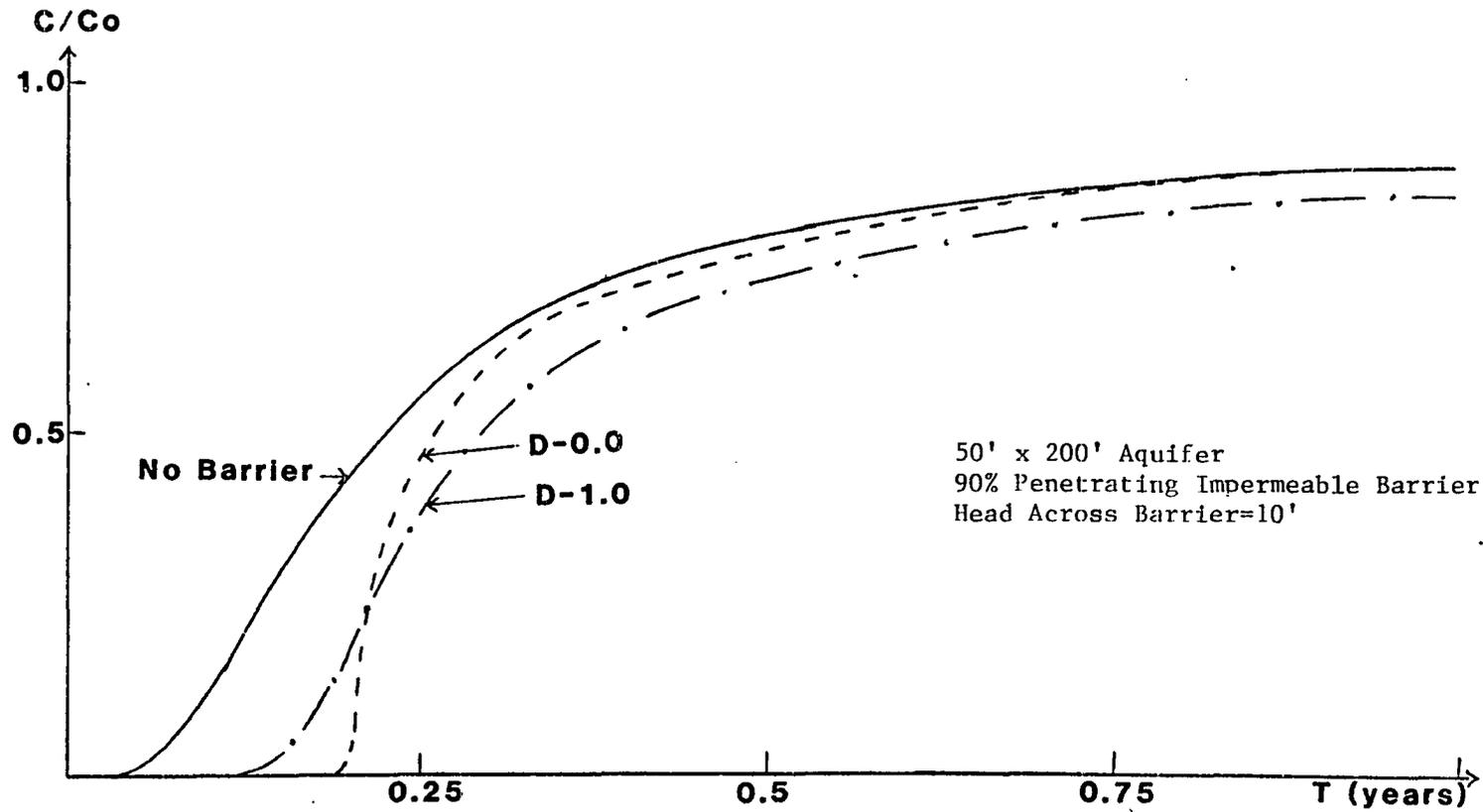
Figure V-18: Pollutant Breakthrough Curves in 50 Foot Deep Aquifer for Head Difference Comparable to 100 Foot Deep Aquifer.
