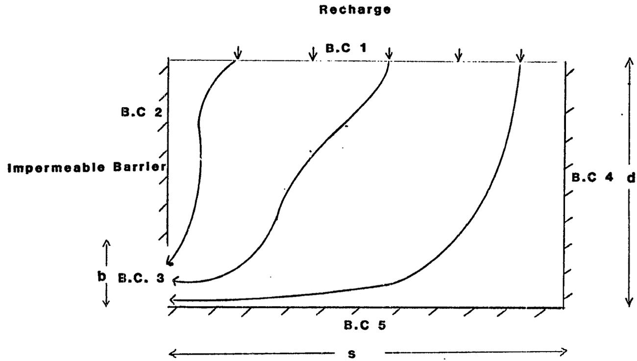
Figure IV-1: Flow of Contaminated Recharge Under an Impermeable Barrier.
