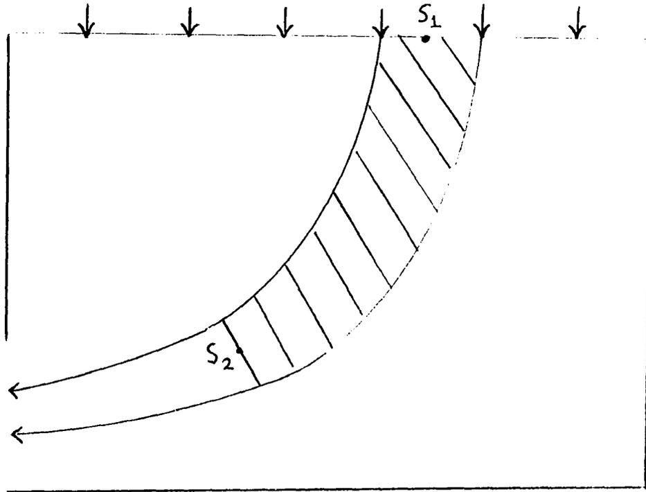
Figure IV-2: Illustration of Plug Flow.
