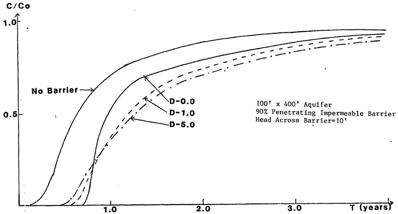
Figure V-15: Pollutant Breakthrough Curves for 100 Foot Deep Aquifer.
