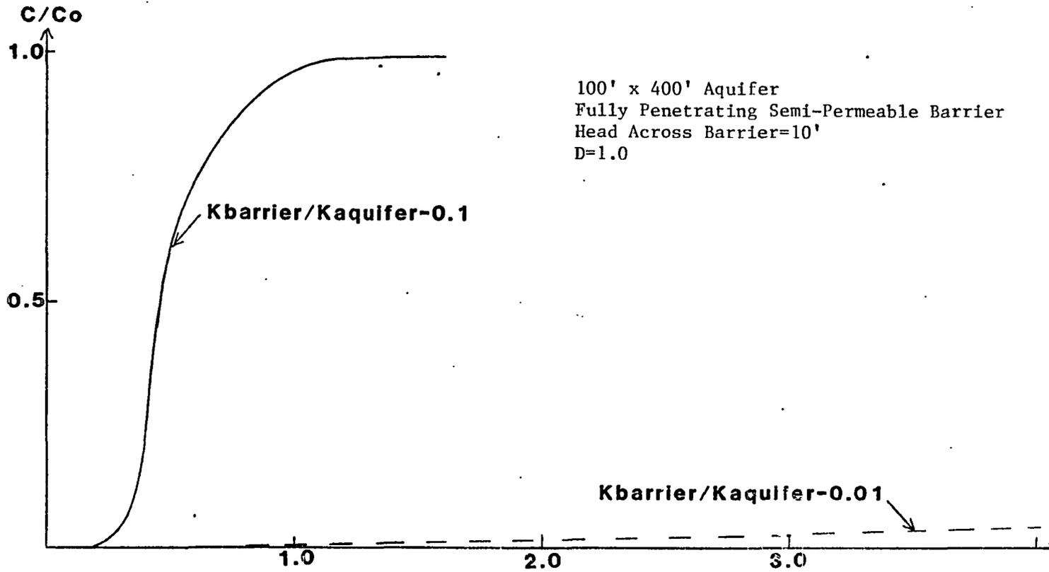
Figure V-25: Pollutant Breakthrough Curves Adjacent to a Semi-Permeable Barrier at 30% Depth.
