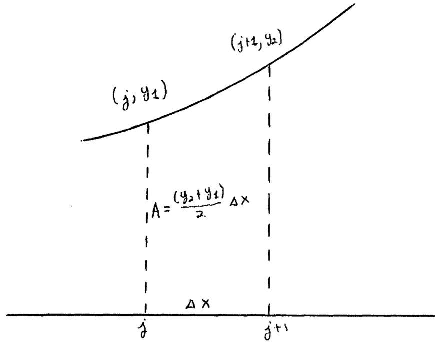
Figure IV-4: Trapezoidal Approximation of Area Under Streamlines.
