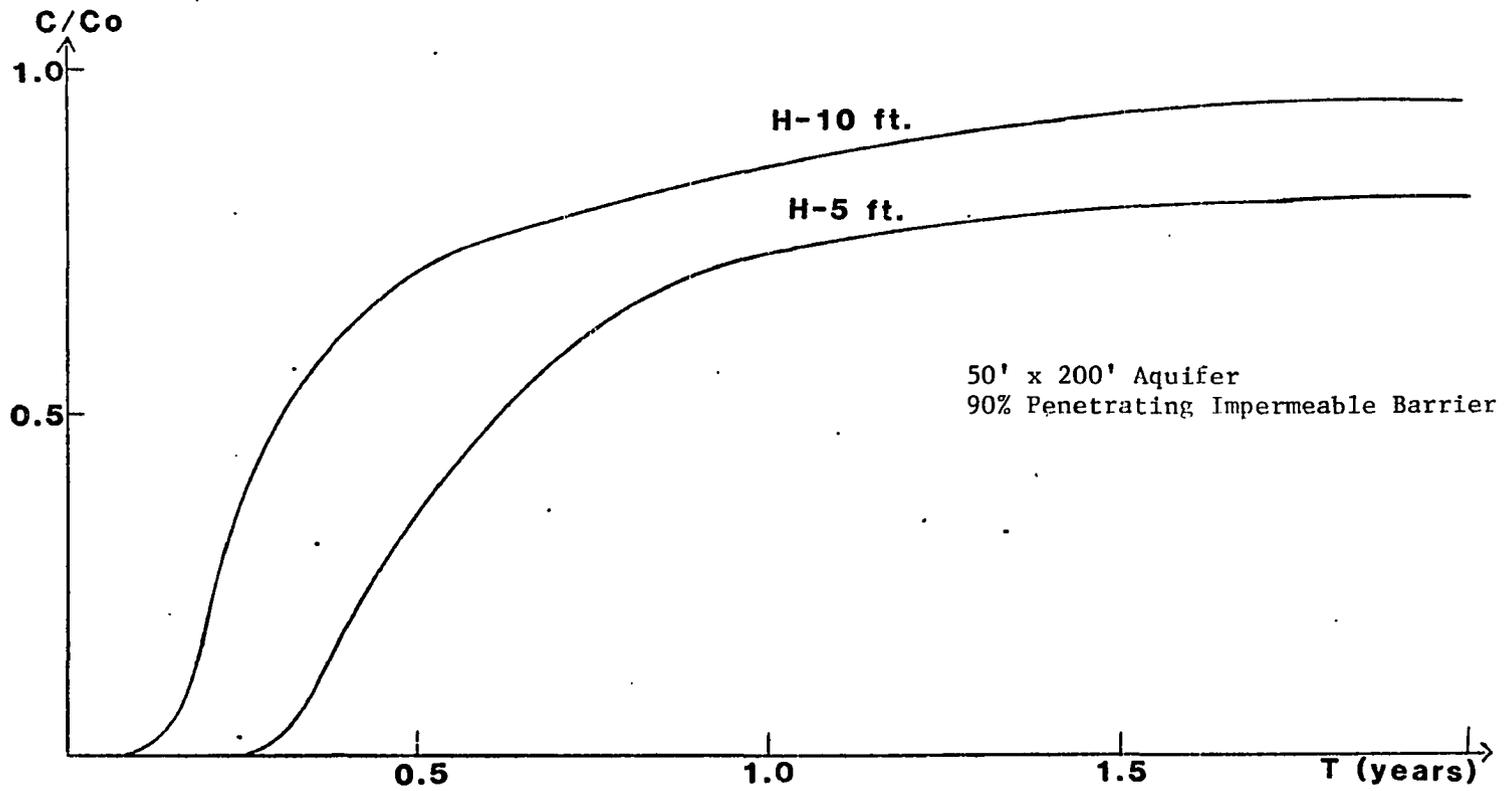
Figure V-20: Pollutant Breakthrough Curves for 50 Foot Deep Aquifer for Two Recharge Rates.
