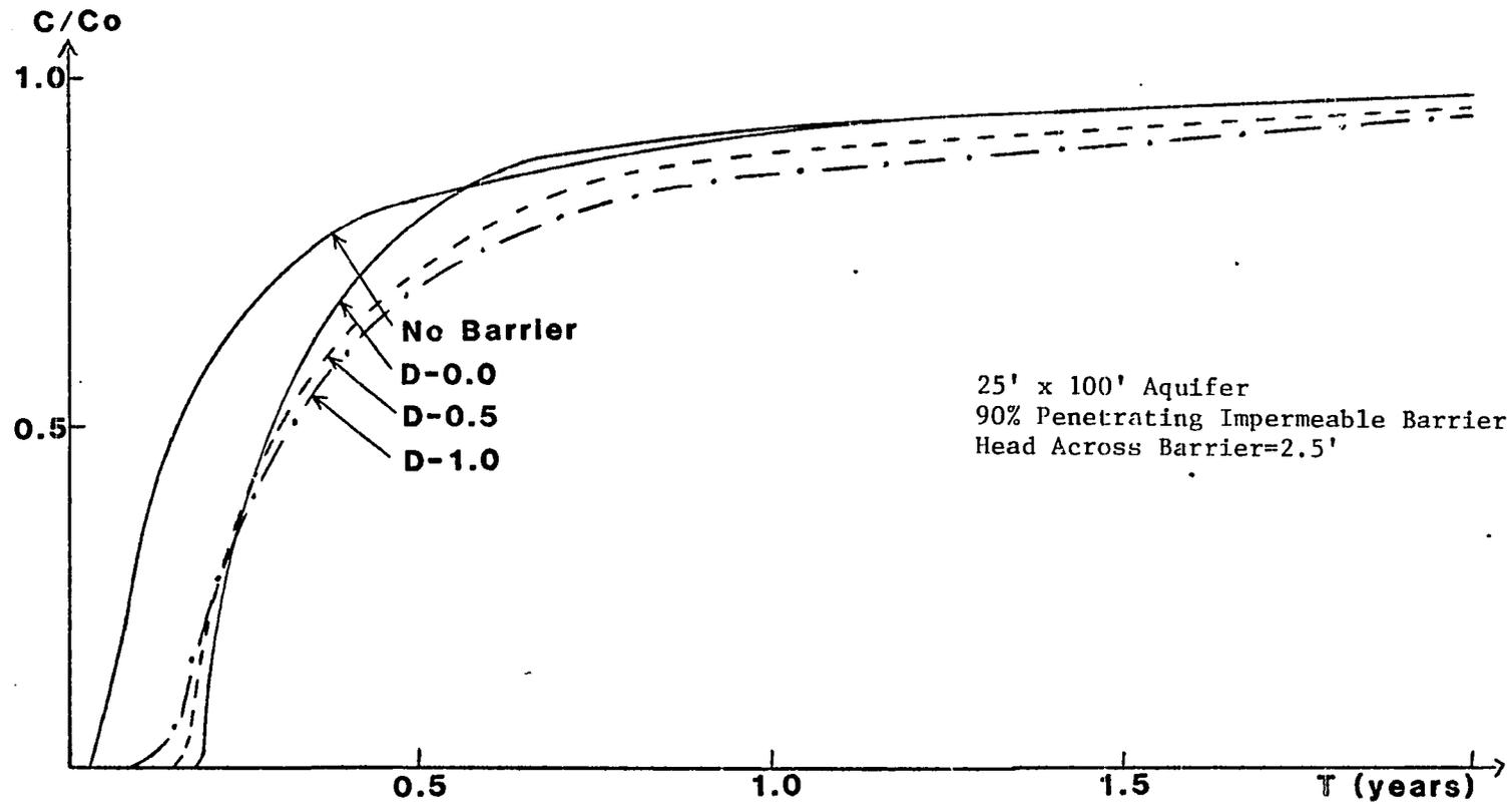
Figure V-17: Pollutant Breakthrough Curves for 25 Foot Deep Aquifer.
