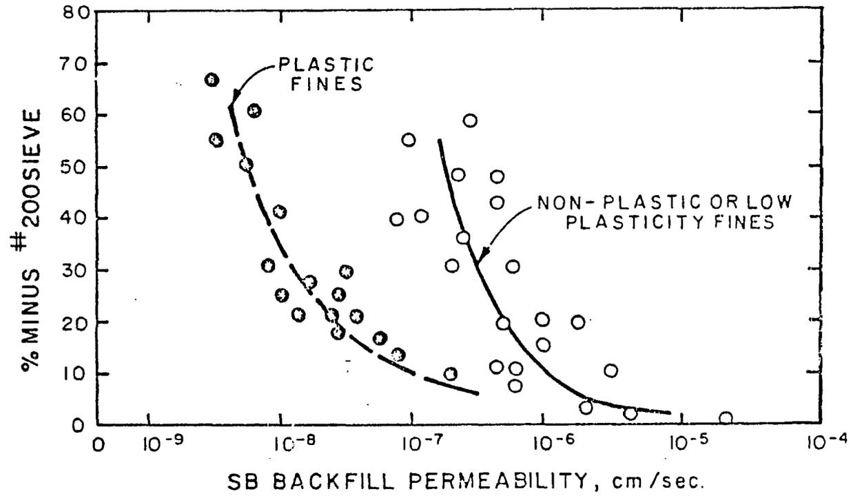
Figure III-5: Permeability of Soil-Bentonite Backfill Related to Fines Content (Ryan, 1980).
