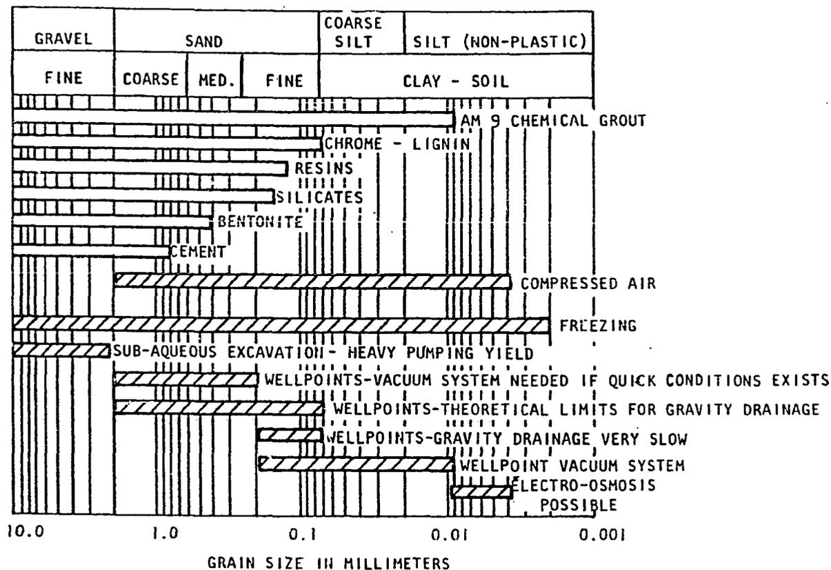
Figure III-1: Soil Gradation Limits for Grout Injection (from American Cyanamid Company).
