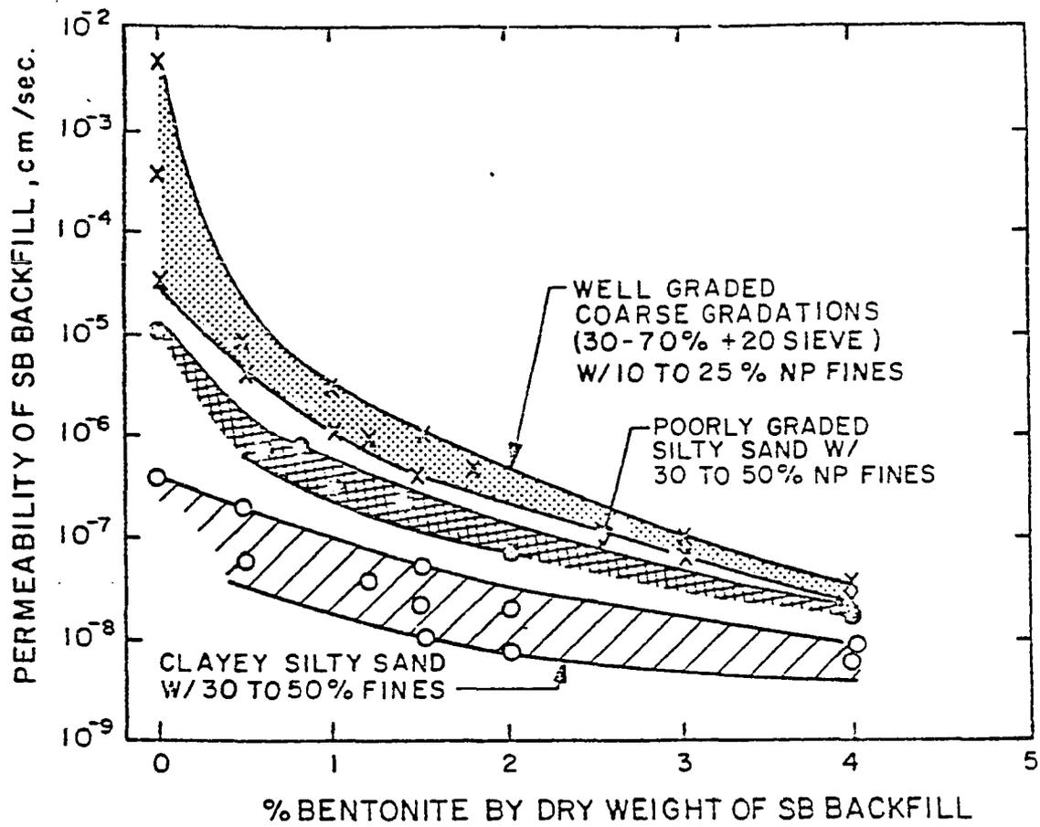
Figure III-4: Relationship Between Permeability and Quantity of Bentonite Added to Soil-Bentonite Backfill (Ryan, 1980).
