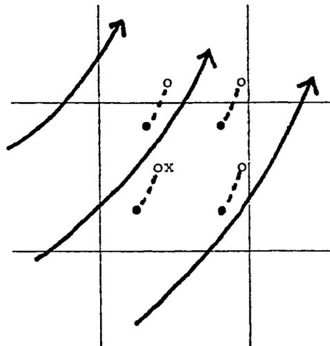
Figure II-2: Finite-Difference Grid Showing Reference Particles.
