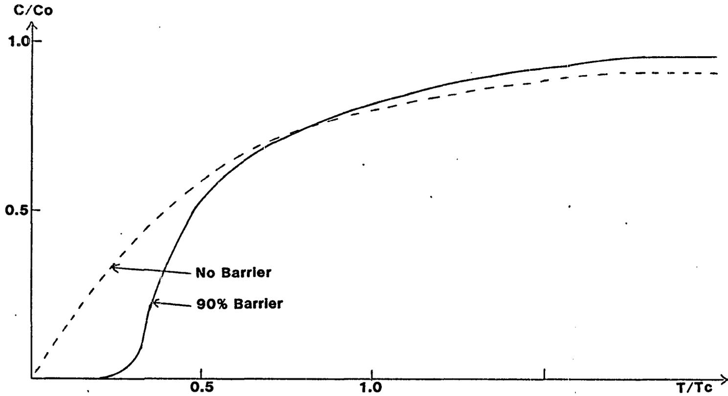
Figure V-11: Pollutant Breakthrough Curves for No-Barrier and 90% Barrier In Horizontally Conductive Soil.
