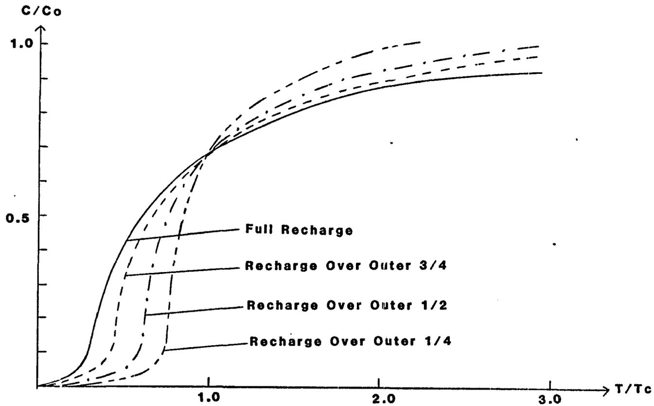
Figure V-8: Pollutant Breakthrough Curves for 90% Penetrating Barrier at Variable Recharge Lengths.
