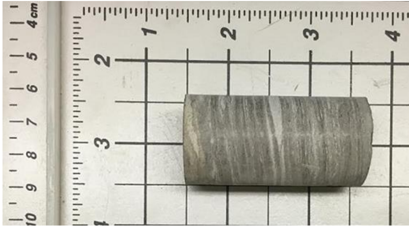
Figure 20. Mancos PAB specimen before testing
