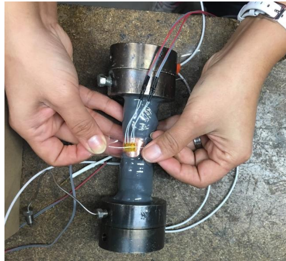
Figure 19. Strain gauges installation
