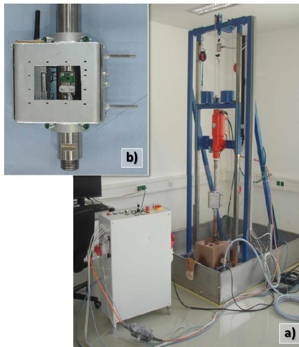
Figure 2.11: a) Laboratory scale rig b) Vibration sensor (Esmaeili et al. 2012)
