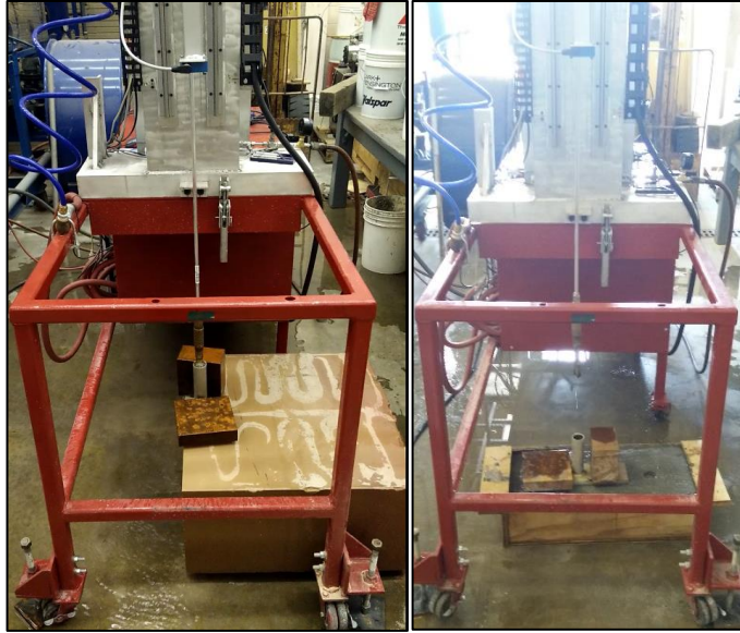
Figure 3.9: Rock sample on left is soft sandstone and on the right is the hard sandstone
