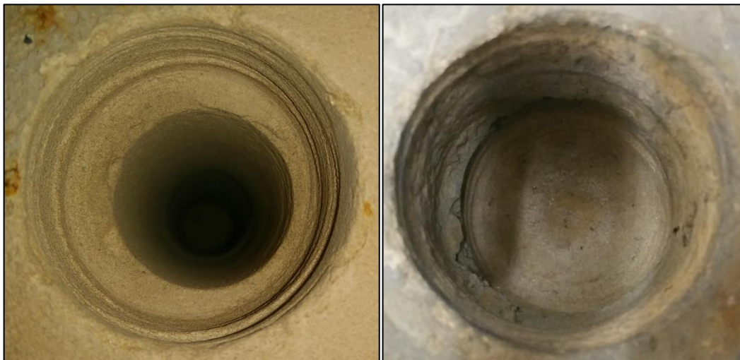
Figure 3.9: Rock sample on left is soft sandstone and on the right is the hard sandstone
