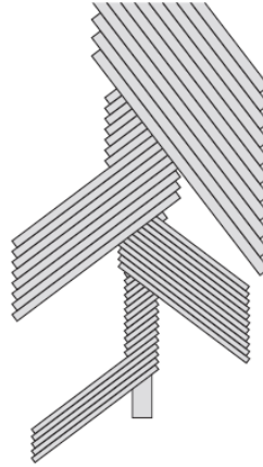
Figure 17. String stiffness schematic used in the setup by Kapitaniak, et al. (2015).
