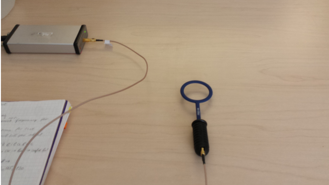
Figure 4.3: The setup for measurements when laptop from Figure 4.1 was taken out of the room.
