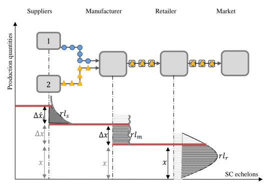
Figure 4-3: Flow depreciation in the forward SC.
