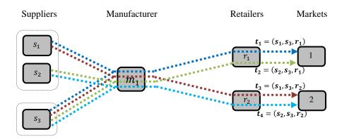
Figure 5-1: Potential paths available in the structure of a sample forward SN.
