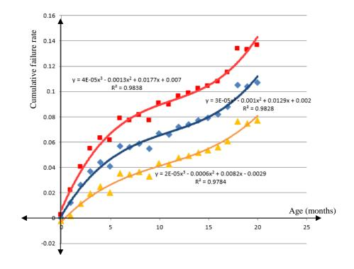
Figure 5-6: Failure rate of the first component with respect to age.
