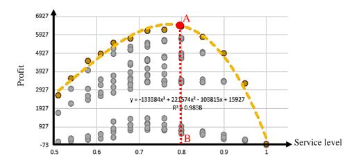
Figure 6-3: Profit of the first supply path with respect to the service level.
