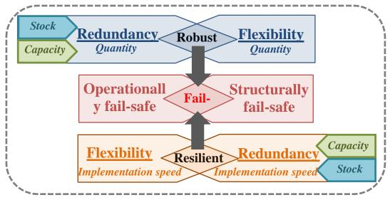
Figure 7-4: Architecting fail-safe systems.
