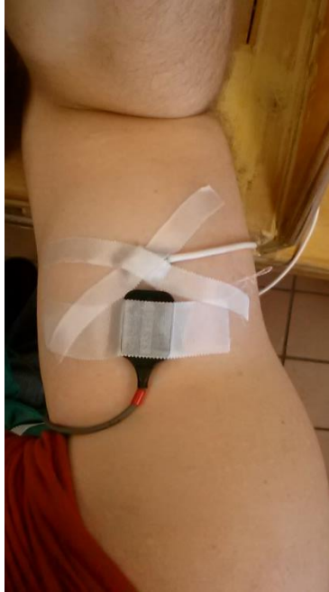
Figure 8. An example of the sensor placement on the BB. On the BB muscle the MMG sensor was located most distal, while the EMG sensor was located most proximal to the shoulder attachment.
