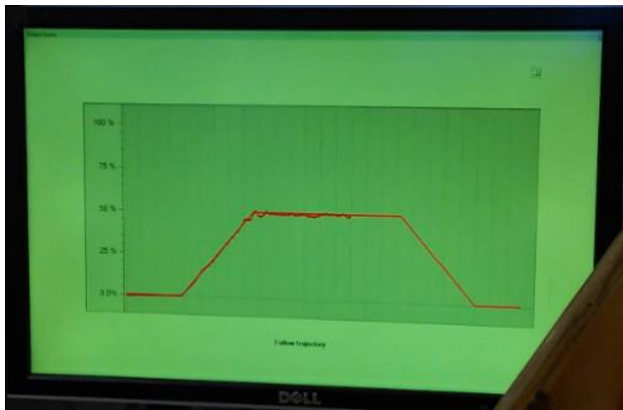
Figure 6. An example of the trapezoid template used for the submaximal isometric muscle actions. Visual feedback of the subject's real time force level was overlaid on the screen as the subject attempts to match the template.
