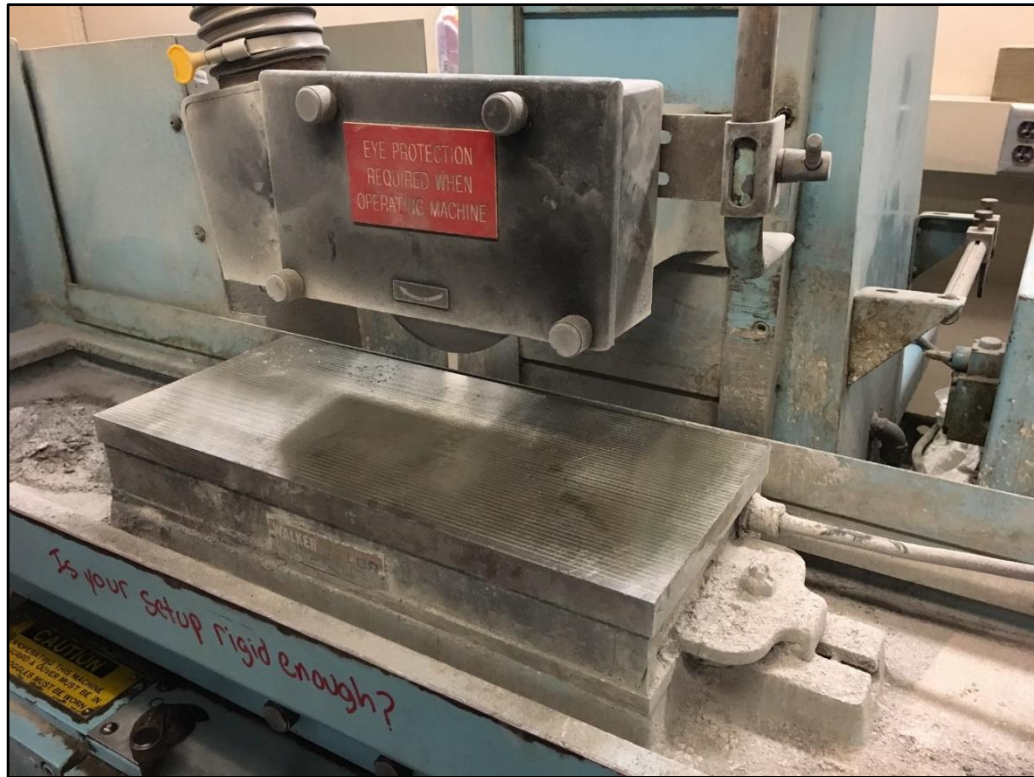
Figure 14. Core polishing machine.
