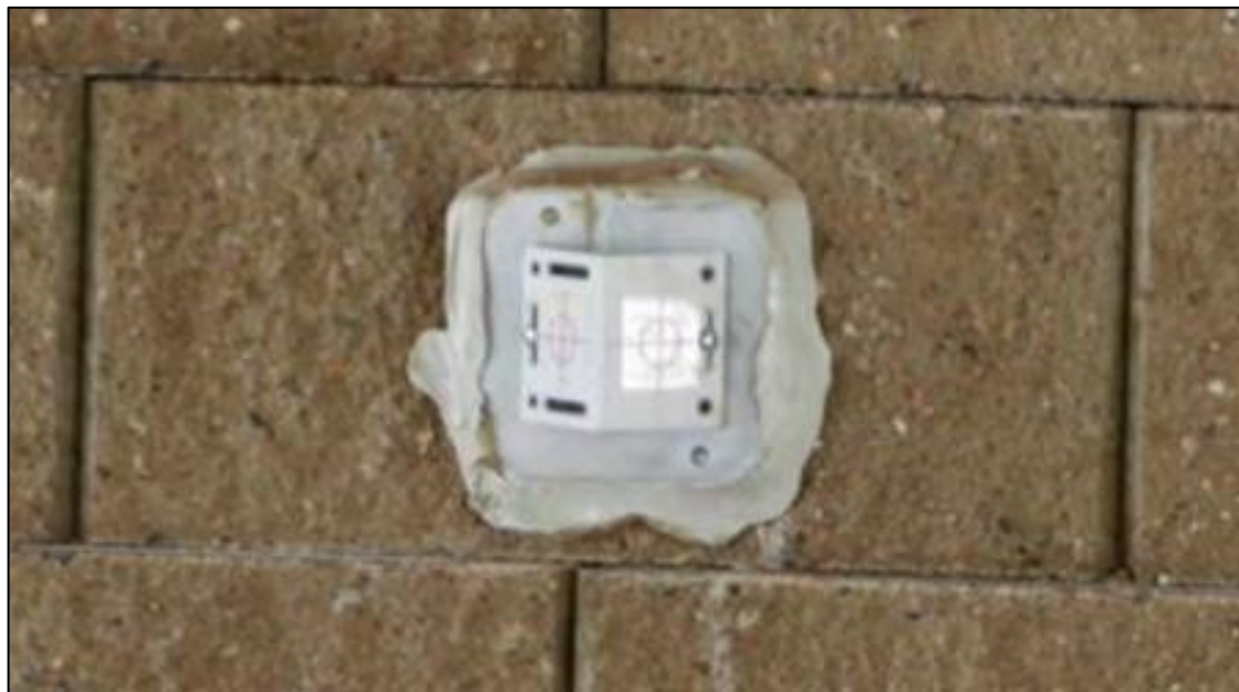
Figure 34: Surveying reflective target installed on abutment wall for STH 40 Bloomer Bridge (Garnier-Villarreal et al. 2014)
