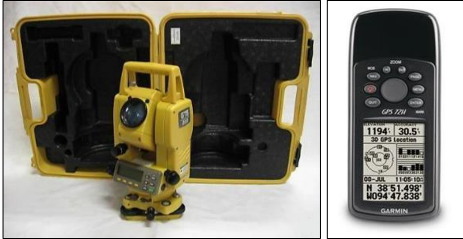
Figure 85: (a) Total Station Topcon GTS-211D used in this study to survey and monitor the deformations of GRS-IBS and conventional bridges; (b) GPS Garmin - 72H
