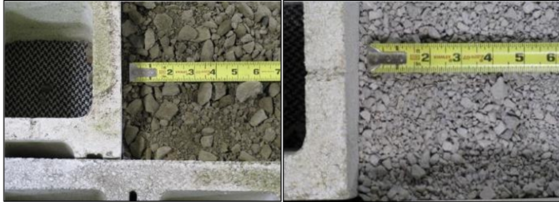
Figure 3: (a) well-graded 21-A gravel; (b) Open-graded AASHTO No. 89 gravel (Adams et al. 2012)
