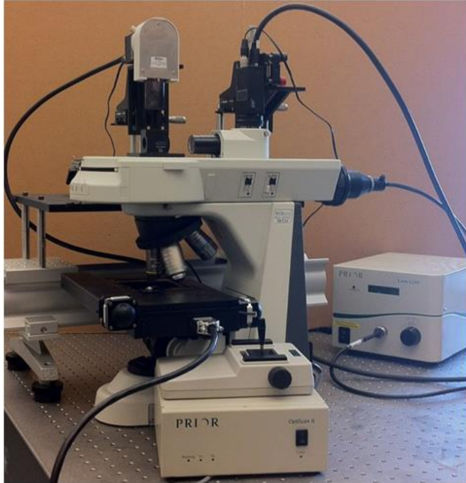
Figure 19 A photo of the duo-color fluorescence microscope imaging system
