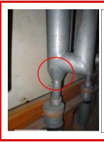
PICTURES OF MOLLER OP. 5819 IN THE PHILADELPHIA CONVENTION CENTER (Left) No detail was left unturned; the ingeniously built miters on the 32' Bombarde evenly support the weight to prevent the pipes from bowing. (Right) Great Mutation Chorus [2-2/3', 2', 1-3/5', 1-1/3', 1-1/7',
