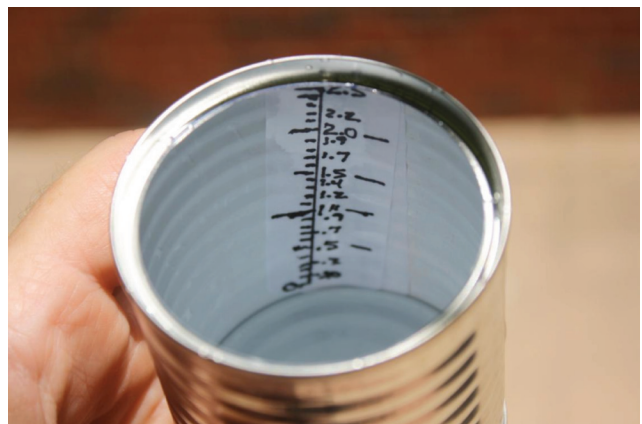
Figure 2. Examples of various catch cups that can be used to conduct the simple irrigation audit and examples of how to mark the side of the catch cups for more accurate irrigation output measurement.
