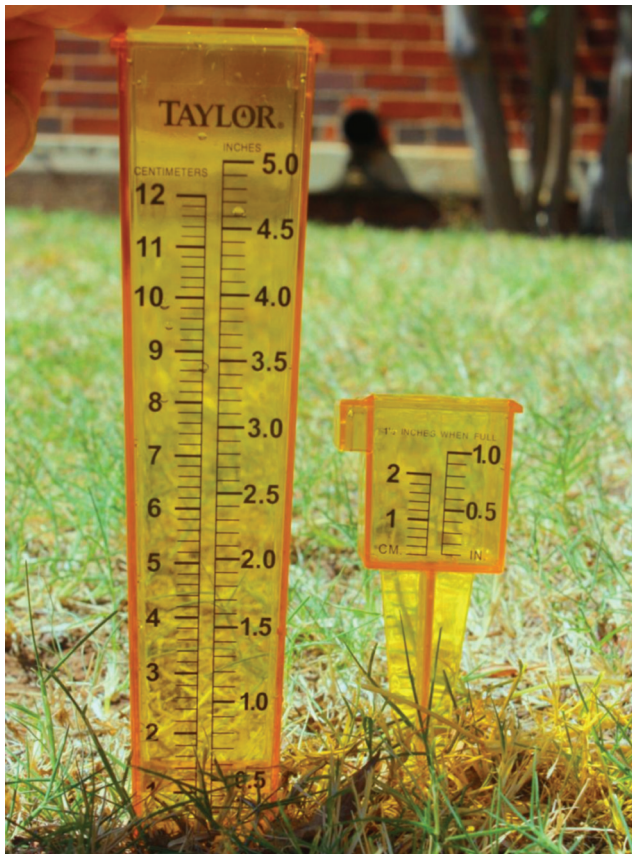
Figure 1. Examples of a short rain gauge (right) that can be used to conduct the simple irrigation audit procedure and a tall rain gauge (left) that should not be used to conduct the simple irrigation audit procedure.
