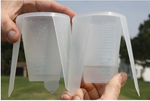
Figure 5. Note the relative uniformity of your irrigation output across the irrigation catch cup grid. If there is too much variation in the sprinkler pattern, you may need to hire a professional to adjust your irrigation system.
