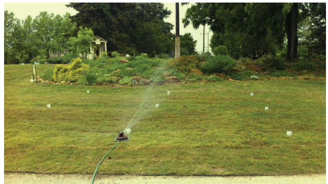
Figure 4. Proper placement of the catch cups in relation to your typical sprinkler location is imperative to obtain accurate irrigation output measurement.
