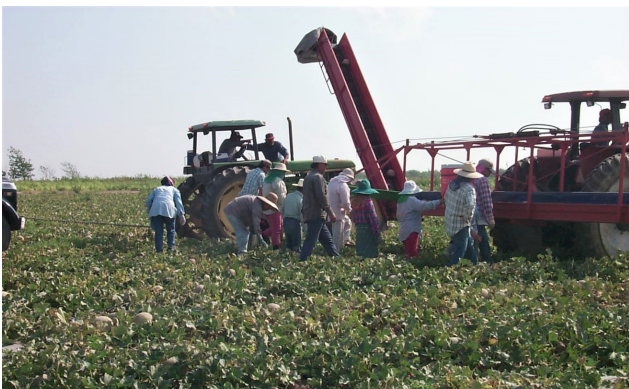
Harvest conveyor to assist hand harvesting.
