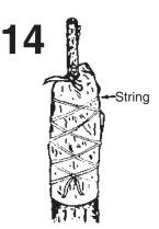
At this point, many grafters use amber shellac to coat the top and sides of the scion down to the polyethylene bag. Make sure the shellac is water based amber or orange shellac.
