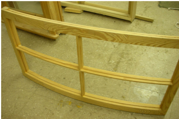
Figure 3. Unfinished curved window made from Southern yellow pine. (Courtesy of Wewoka Window Works)
