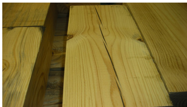
Figure 2. Large cracks on the longitudinal direction of the raw material.
