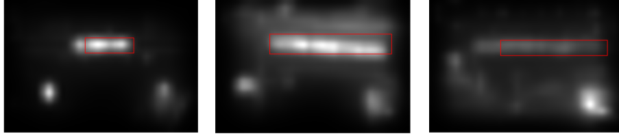
Figure 4.11: GBVS saliency maps calculated on SVT [86] dataset. The red rectangle indicates the ground truth text regions. The left appears to help text localization, the middle produces too much regions, and the right selects non-text regions
