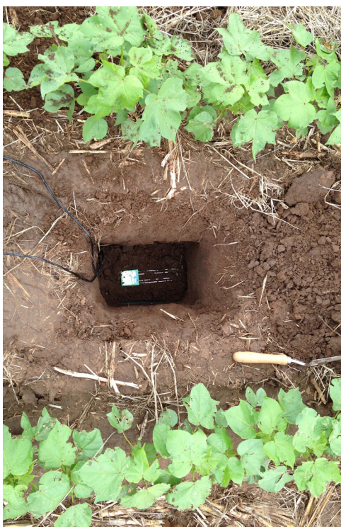
Figure 4. Installing soil moisture sensors at a cotton field near Altus.
