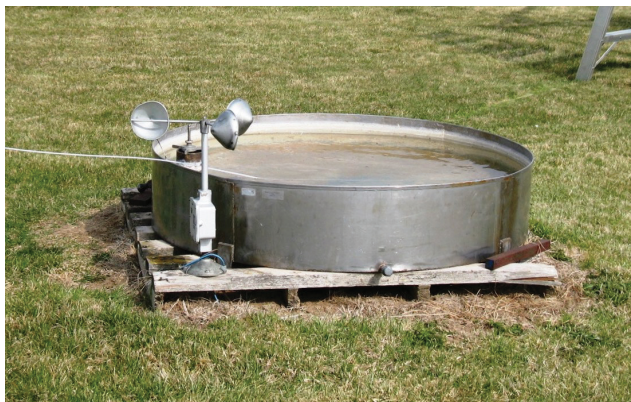
Figure 2. Class A evaporation pan at the USDA-ARS weather station at Kimberly, Idaho.
