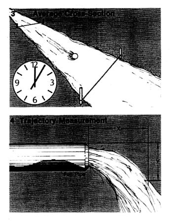
I ne trajectory method of water measurement is a form of velocity area calculations that can be used for determining the rate of flow discharging from a horizontal pipe flowing full. Two measurements of the discharging jet are required to calculate the rate of flow of the water. The first measurement is the horizontal distance, "X", (parallel to the centerline of the pipe) required for the jet to drop a vertical distance "Y" which is the second measurement.
