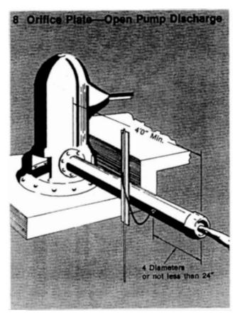
K = a constant dependent upon a combination of pipe size, orifice size and orifice shape, and discharge conditions.
