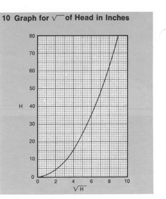
The following graph can be used for determining the "square root" of the head (H) in inches. Having measured the head H using the glass tube and a scale, enter the graph at the left side. Move horizontally to intercept the curve and move downward to determine the square root of H ( $\sqrt{H}$ ).
