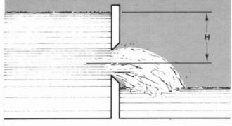
Generally, only one or two measurements are required where the dimensions of the constriction are known. Using these measurements, rate of flow is determined from either a table, a graph, or by calculation. Due to the wide variety of types and sizes of constricting devices, flow tables are not included in this publication. The local County Extension Director or local USDA office can obtain such tables or graphs.
