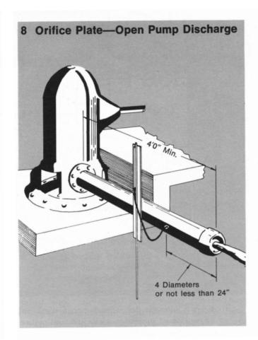
the flow from the orifice discharges entirely into air or "fully submerged" where the downstream water surface is above the top of the orifice and the flow discharges into water. Avoid orifices that do not flow free or are not completely submerged.
