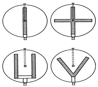
Figure 5. Common platterns for aeration ducts.
