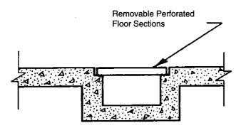
Figure 4. Flush-floor ducts are usually rectangular in cross-section.
