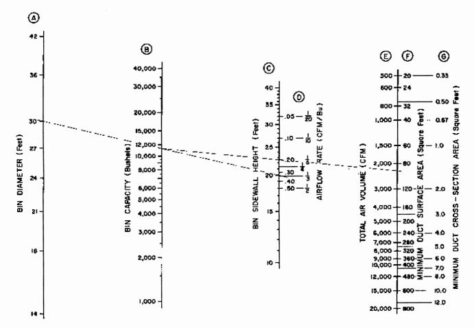
Nomograph 1. Bin capacity, total air volume and minimum duct areas.
