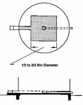
Figure 2. A partially-perforated floor system.
