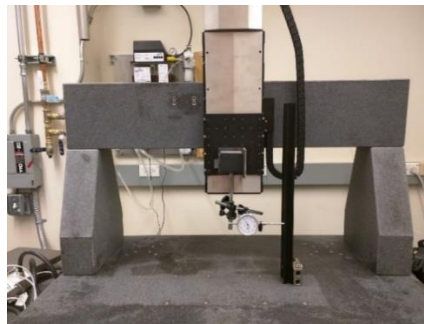
Figure 3.4 Alignment of Z-axis
