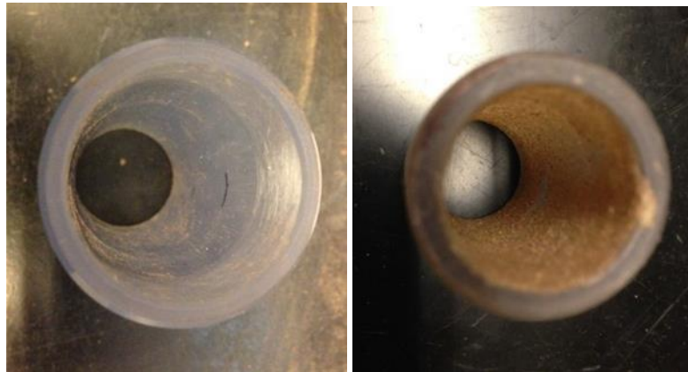
Figure 7. Smooth walled polyvinyl chloride pipe (left) and sand adhered to the inside pipe wall to increase the roughness of the pipe (right).
