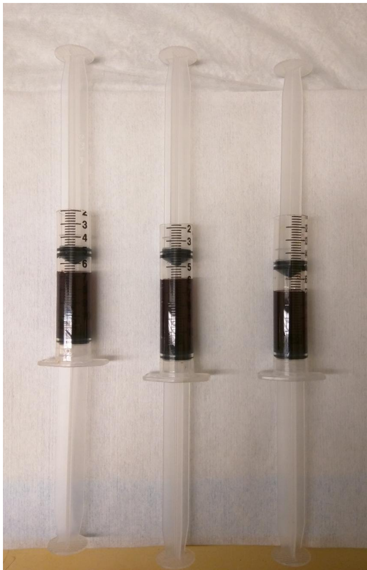
Figure 3.1: Multiple wet ‘sol’ gels after mixture of vanadium tripropoxide and water/acetone solution; subsequently left for aging for 5 days.
