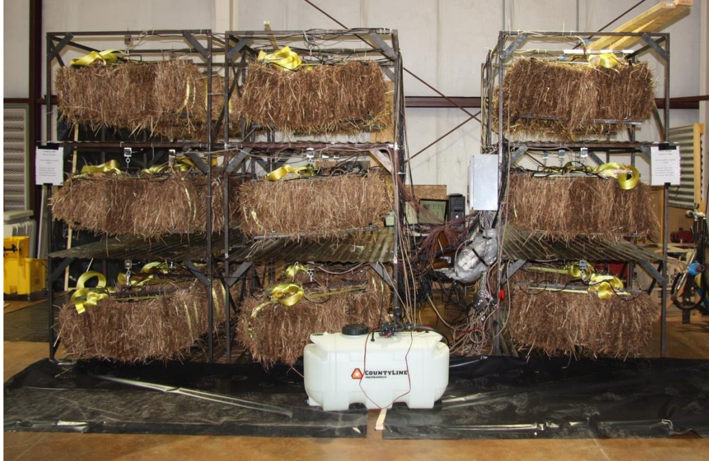
Figure 3.7. Picture of the automated watering system with all 27 bales in storage
