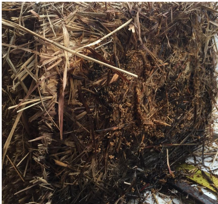
Figure 3.16. Bale 9 (3% fungal loading, 81 d), no visible fungal growth, shows deterioration
