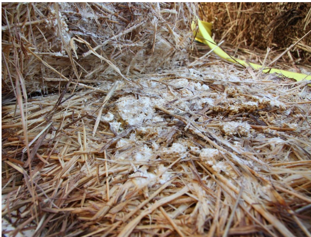
Figure 3.13. Bale 17 (3% fungal loading, 53 d), visible fungal growth (white)
