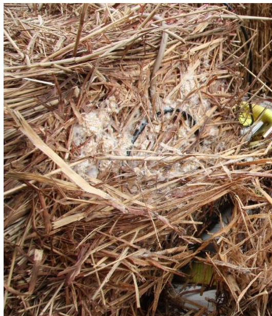
Figure 3.9. Bale 24 (2% fungal loading, 25 d), fungal growth visible (white)
