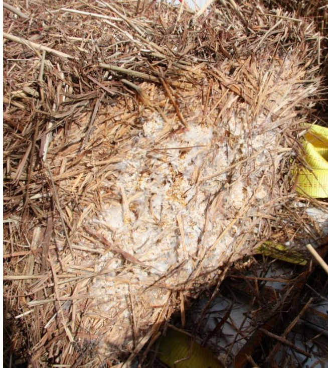
Figure 3.10. Bale 25 (3% fungal loading, 25 d), fungal growth visible (white)
