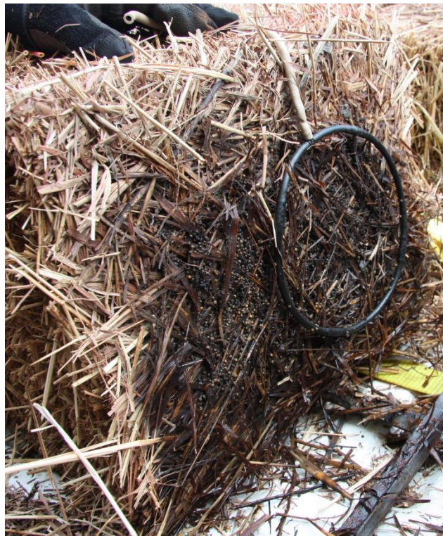
Figure 3.8. Bale 19 (0% fungal loading, 25 d), deterioration of switchgrass is evident
