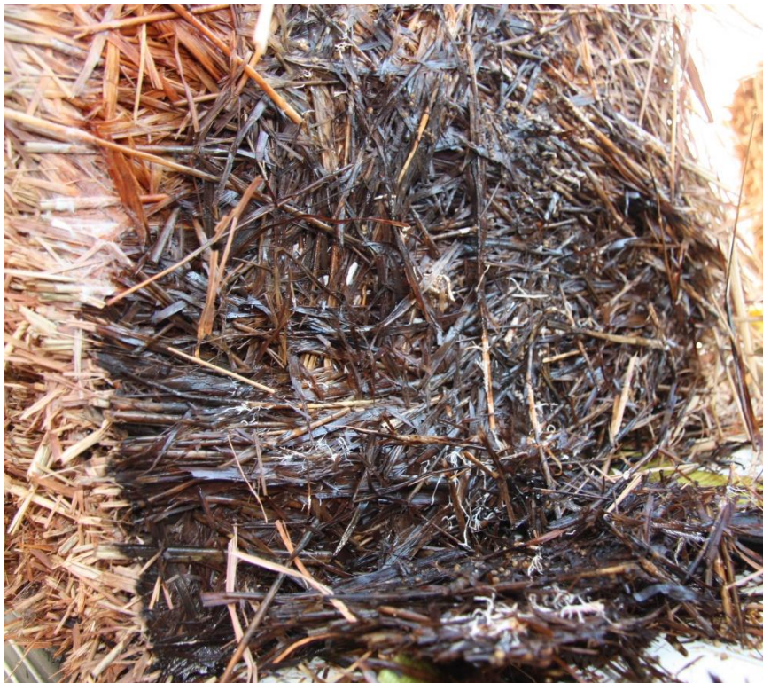
Figure 3.11. Bale 12 (0% fungal loading, 53 d), deterioration of switchgrass is apparent
