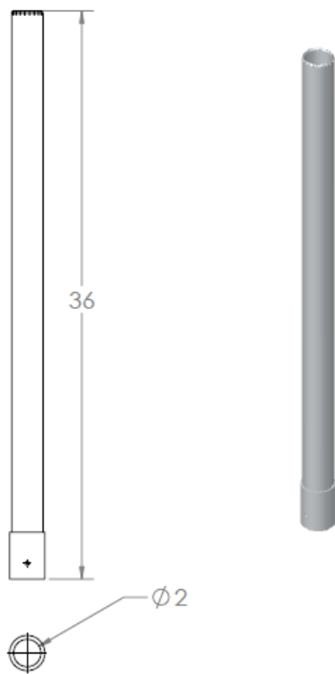
Figure 6.20. Core sampling tube SolidWorks drawing, dimensions in inches
