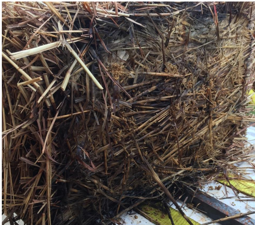
Figure 3.15. Bale 6 (2% fungal loading, 81 d), no visible fungal growth, shows deterioration
