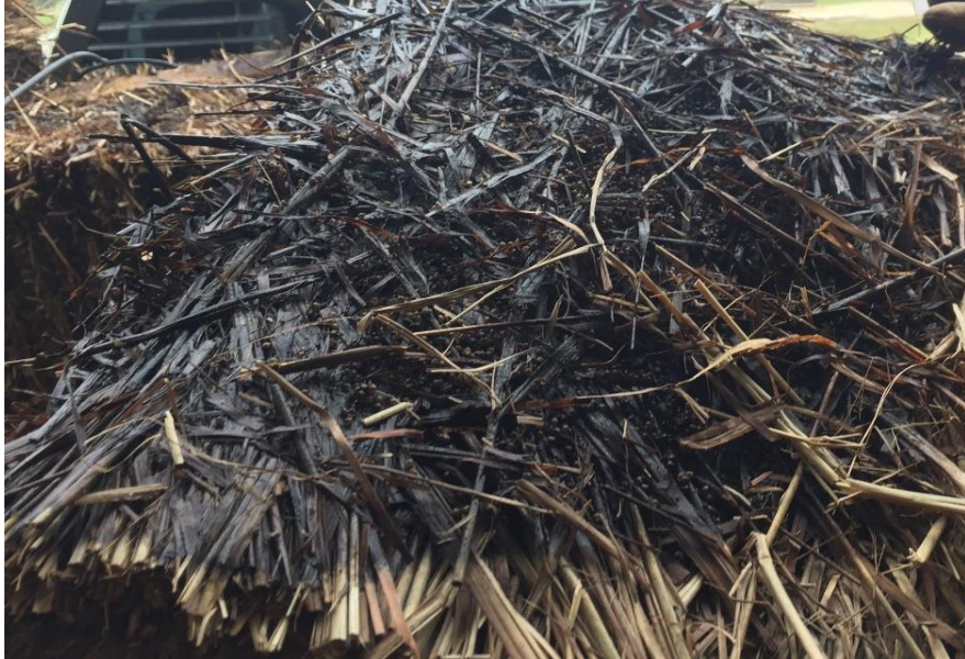
Figure 3.14. Bale 2 (0% fungal loading, 81 d), deteriorated switchgrass
