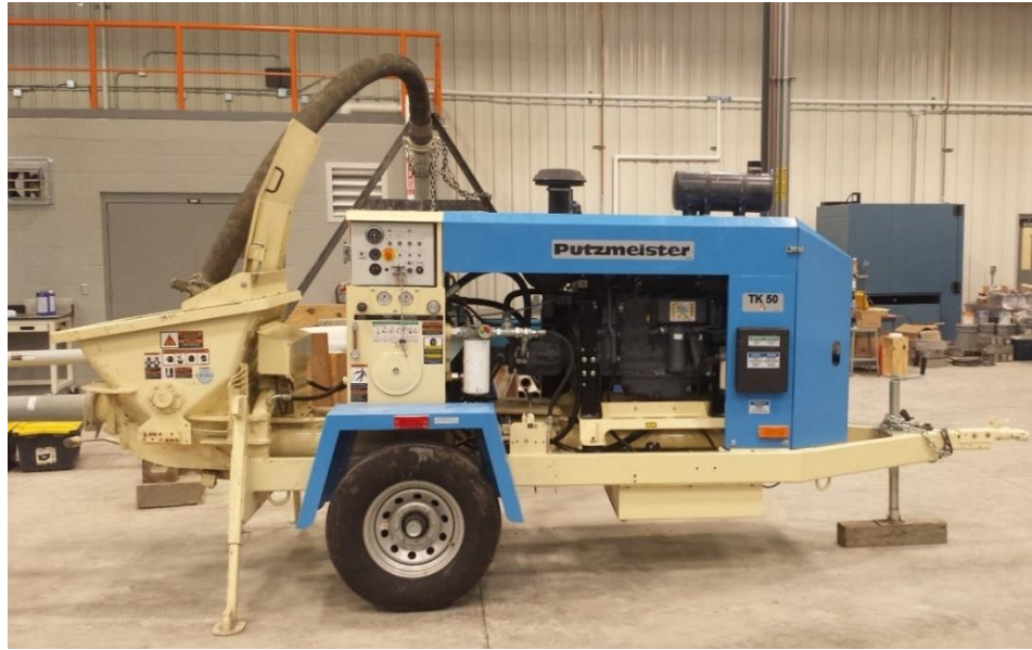
Figure 3: The concrete pump used in this work (Putzmeister TK 50).
