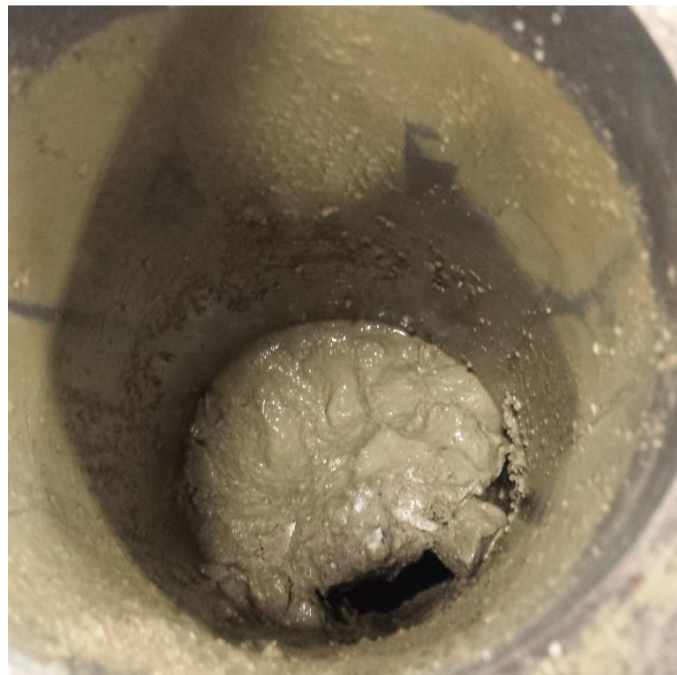
Figure 21: Concrete with 24% fine sands has insufficient mortar to coat the pipeline, causing a jam.
