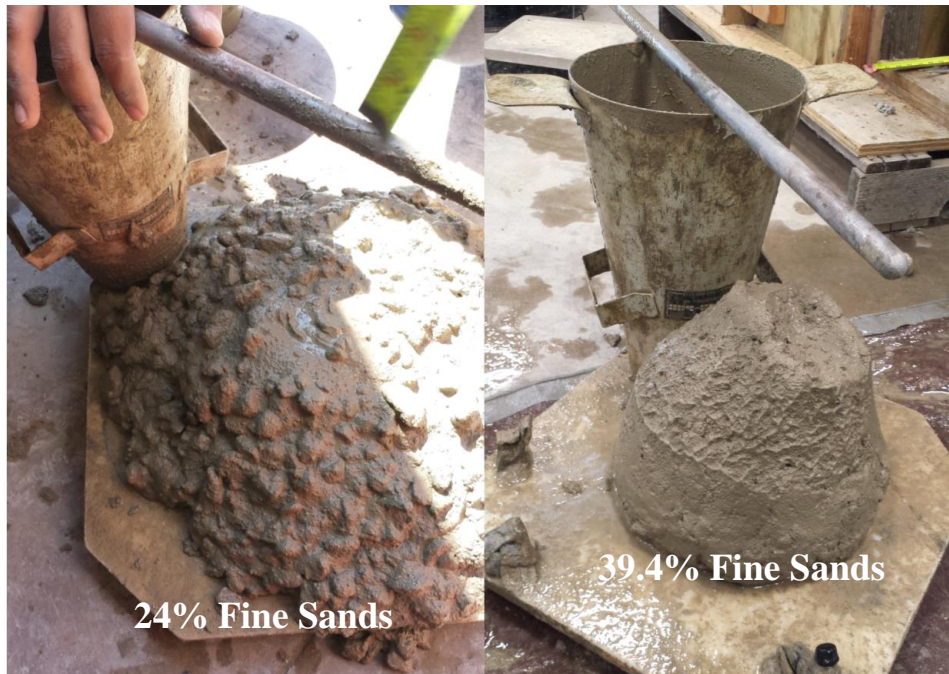
Figure 20: Concrete with 24% fine sands breaks apart when the slump test is conducted.
