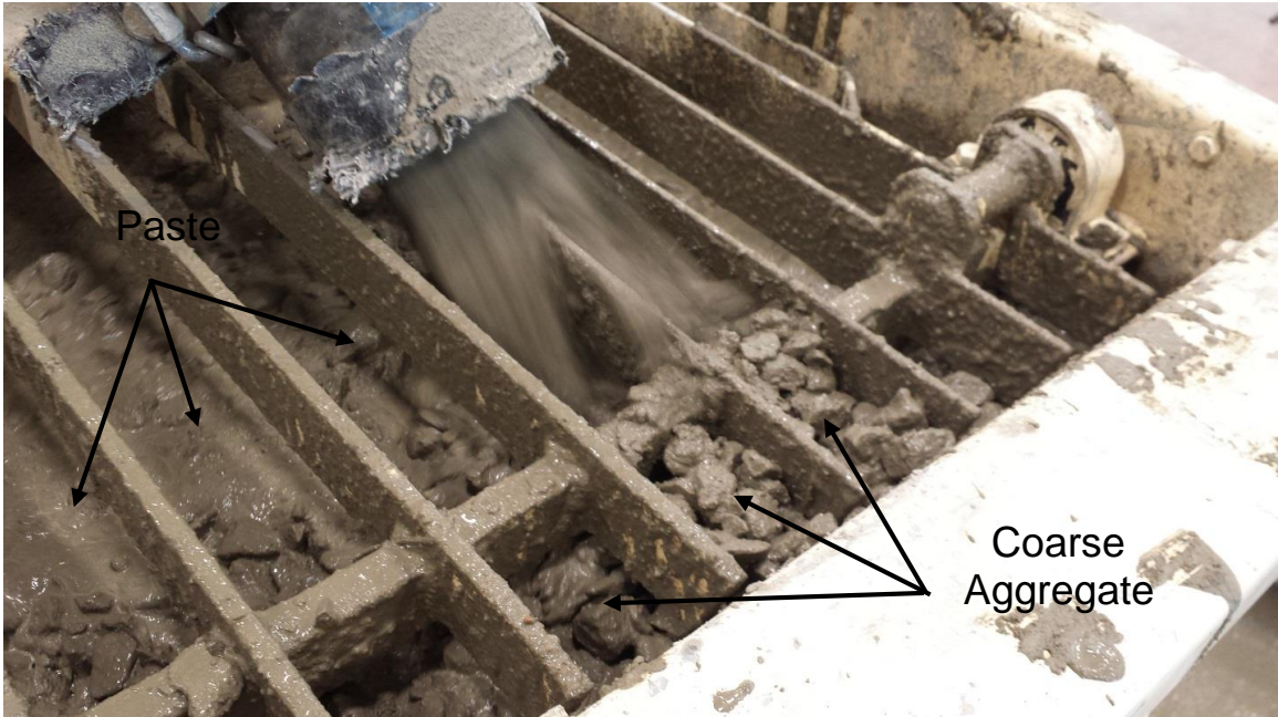
Figure 17: Coarse aggregate exiting the pipeline and showing segregation.
