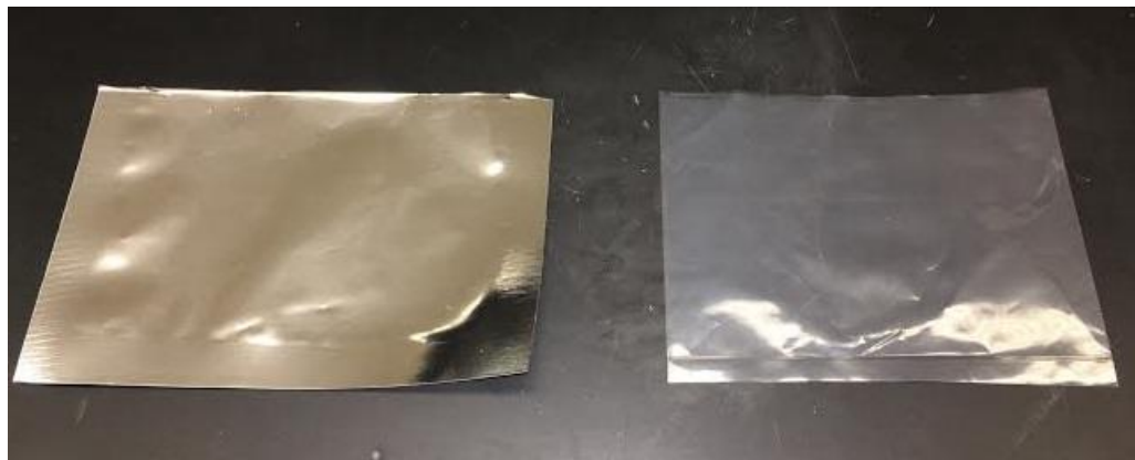
Figure 9. Metallized (left) and plastic (right) packaging materials
