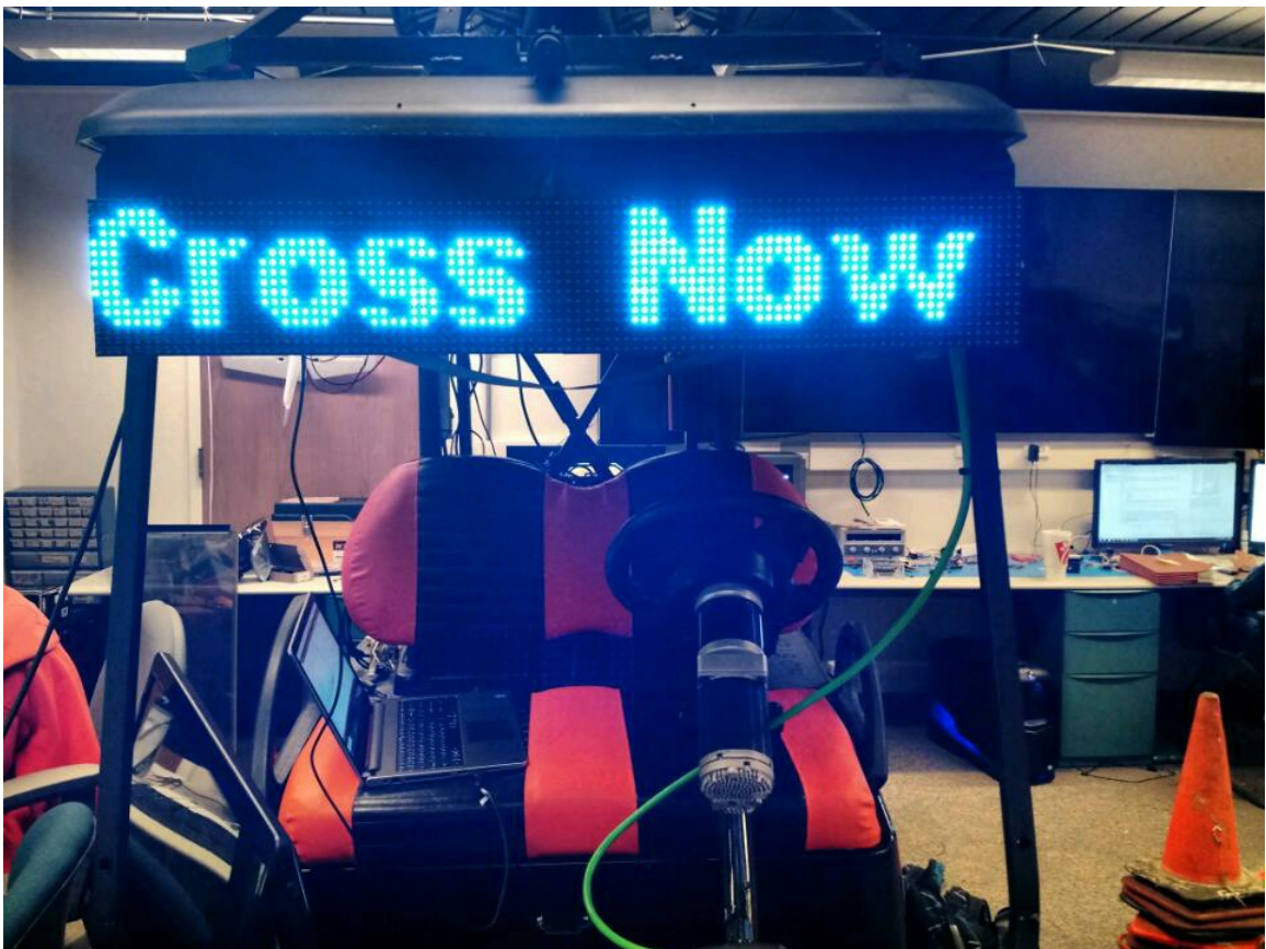
Figure 5.5: Example Visual message displayed by the Intent Communication System
