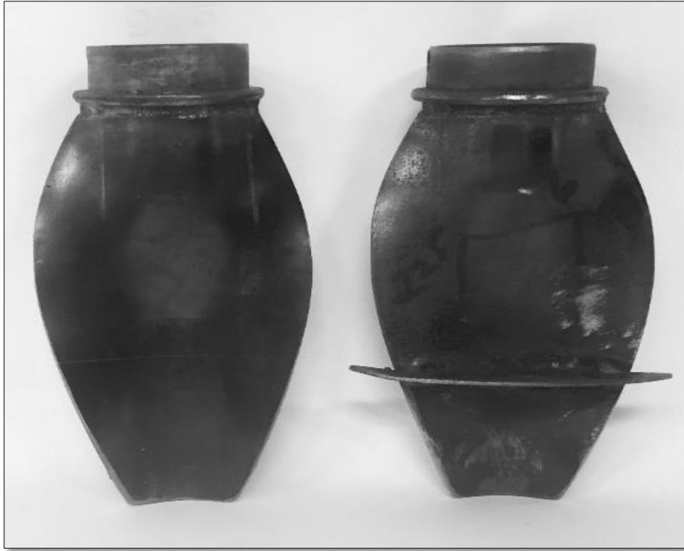
Figure 2. Conventional and tip with a welded stop.
