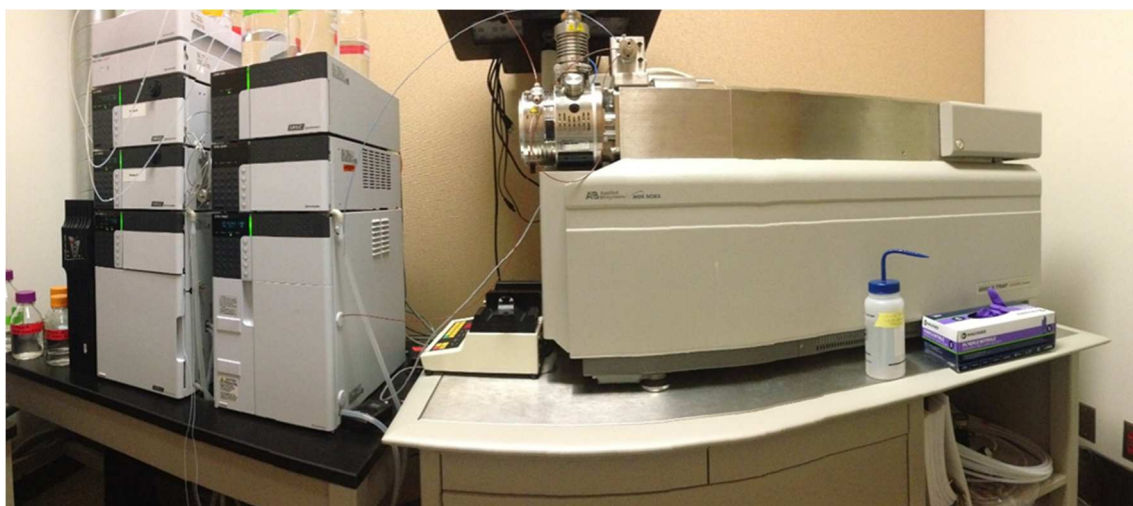
Figure 3. Photograph of LC-MS/MS used in method development.
