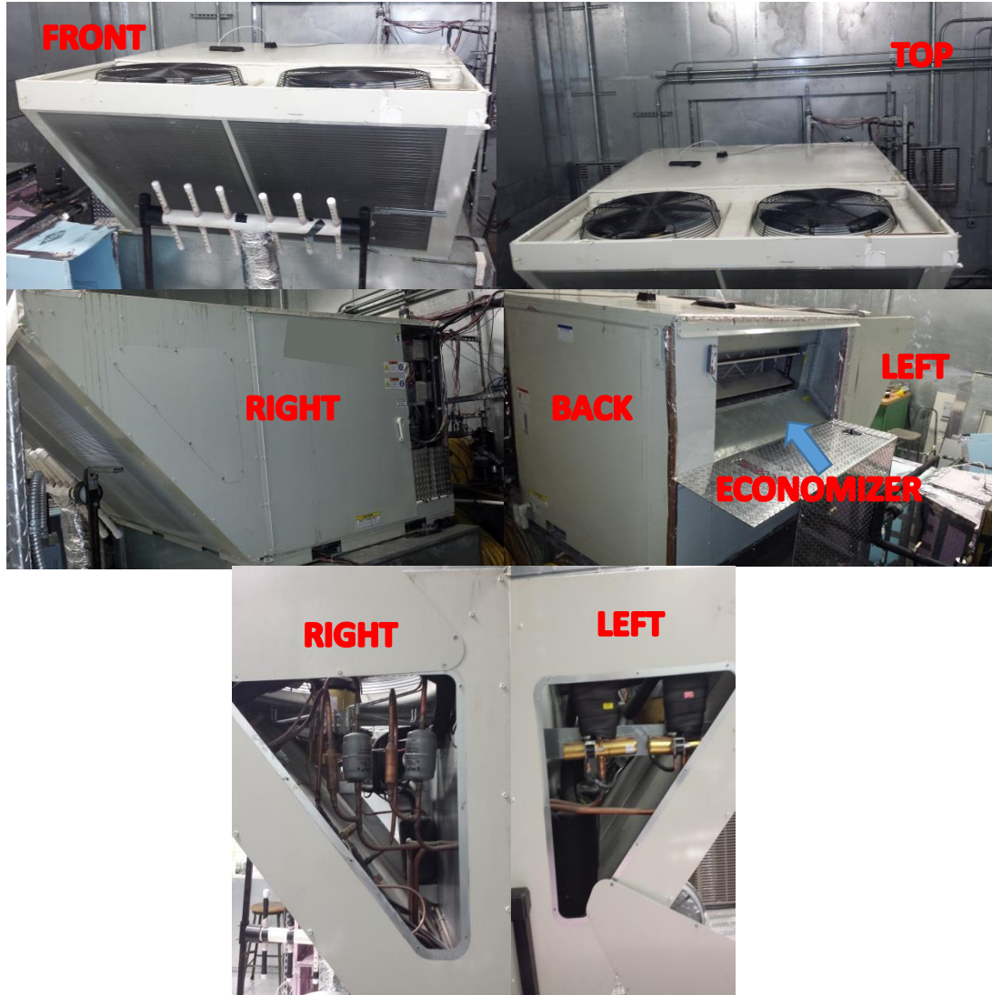
Figure 8: Photos of the 15-ton nominal capacity air-to-air RTU used in the present work and installed inside OSU psychrometric chamber
