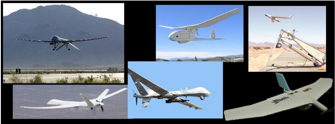
Figure 4: Examples of Propeller Driven UAVs (From Top Left, Clockwise: Predator, Raven, Scan Eagle, Wasp III, Reaper, Altair)
