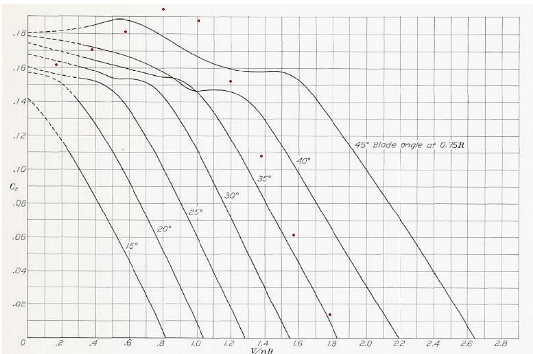
Figure 67: Thrust Coefficient Chart for Propeller 5868-9, Clark-Y, 3 Blades (NACA Report 640) with PROPDES Predictions
