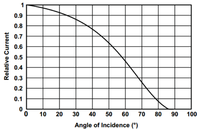
Figure 9. PV Output Current vs Angle of Incident [16]
