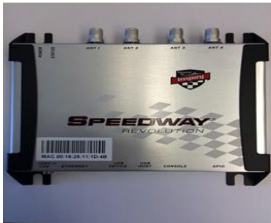
Impinj Speedway Revolution R420 UHF RFID Reader (4 Port) [The WISP can communicate with commercial-off-the-shelf RFID readers, and is powered by the carrier signal emitted by the reader.]
