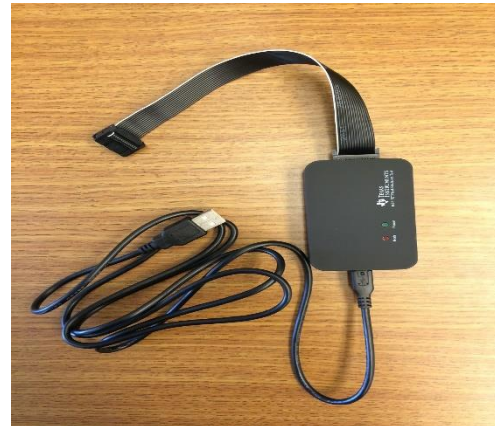
WISP 5.0 Hardware and MSP-FET430UIF programming and debugging tool
