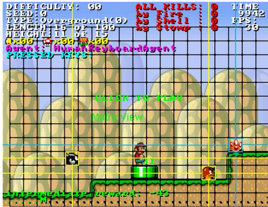
Figure 15 Enemy input information: Input feature extraction for enemies search the visible grid and returns the enemy's x and y coordinates. Enemies that Mario can jump on are represented by the yellow square (the Bullet and the Goomba) and enemies that Mario cannot jump on are represented by the blue square (the Spiny Shell)
