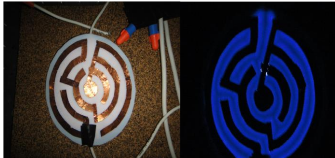
Figure 2 (a) Schematic of Surface Dielectric Barrier Discharge (SDBD); (b) Plasma discharge for a Surface Dielectric Barrier Discharge; (c) Volumetric DBD plasma generation [184].
