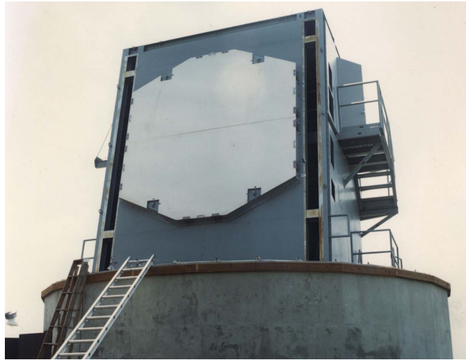
Figure 2.4: Phased-array antenna for the National Weather Radar Testbed in Norman, OK. This antenna is composed of 4352 radiating elements, and it can electronically steer the beam to \pm 45^\circ . The 3-dB beamwidth is 1.5^\circ at broadside (the direction that is normal to the plane of the array) and widens to 2.1^\circ when steered to 45^\circ . The ability to electronically steer the beams allows for adaptive scanning strategies that focus on regions of interest to provide faster updates (Zrnić et al. 2007).
