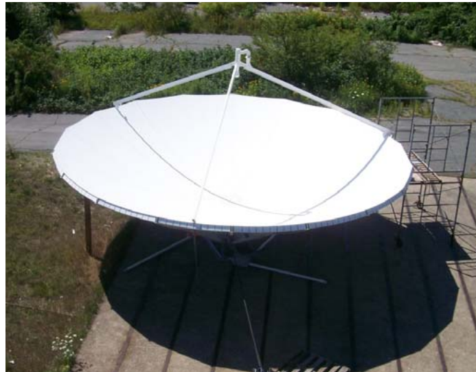
Figure 2.2: S-band parabolic reflector antenna used by the WSR-88D (Ice et al. 2015). This dish antenna has a diameter of 8.53 m and produces a beam with 0.93^\circ 3-dB beamwidth with low sidelobes. The antenna is to be rotated in azimuth and tilted in elevation to allow the narrow beam, also referred to as a “pencil” beam, to scan an entire volume.
